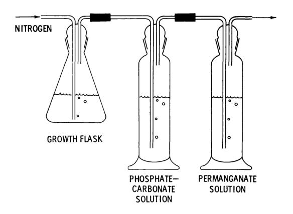
Figure 1. Growth system with mercury traps29
