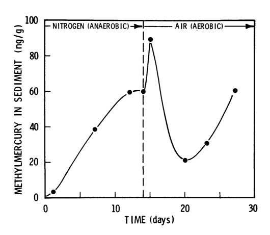
Figure 2. Production of methylmercury in water-sediment systems.
