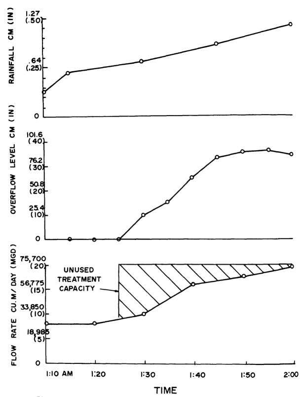
Figure 29. Rainfall, 67th Street overflow level and demonstration system flow rate versus time for Run No. 9
