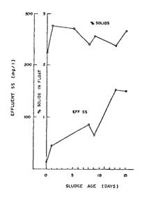
Figure 45. Effluent SS and Percent Float Solids Versus Sludge Age for Bench Scale Tests August 8, 1973 to August 23, 1973
