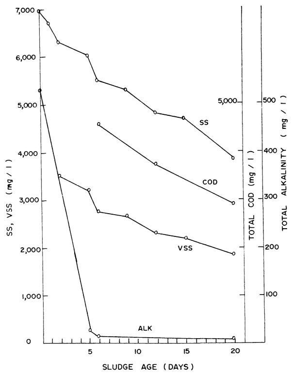
Figure 38. SS, VSS, Total COD, and Total Alkalinity Concentration versus Sludge Age for Bench Scale Tests
