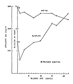
Figure 46. Flotation Test Percent Float Solids and Effluent SS versus Sludge Age for August 28, 1973 to September 19, 1973
