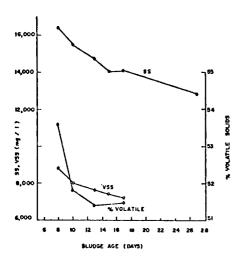
Figure 31. SS, VSS, and Percent Volatile Solids versus Sludge Age for August 18, 1972 to September 11, 1972
