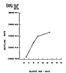
Figure 32. Calculated Surface Overflow Rate versus Sludge Age for August 18, 1972 to September 11, 1972
