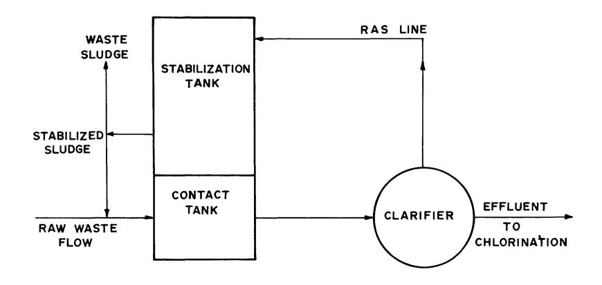
Figure 4. Schematic diagram of contact stabilization process
