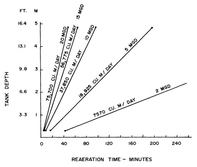
Figure 12. Stabilization tank depth versus reaeration time at various flows
