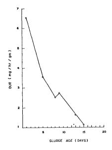
Figure 42. Oxygen Uptake Rate versus Sludge Age for Bench Scale Tests, August 8, 1973 to August 23, 1973
