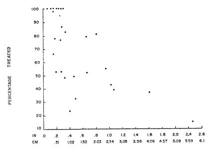
Figure 28. Percentage of overflow treated versus rainfall amounts for 28 events
