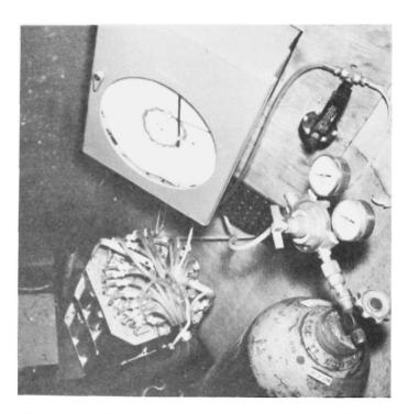
Figure 21. Interior view of monitoring station showing sampling and flow recording instrumentation
