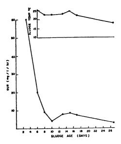
Figure 30. Oxygen Uptake Rate and Sludge Temperature versus Sludge Age for August 18, 1972 to September 1972
