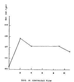
Figure 37. Calculated Sludge Volume Index versus Days of Continuous Flow for July 9, 1973 to July 20, 1973
