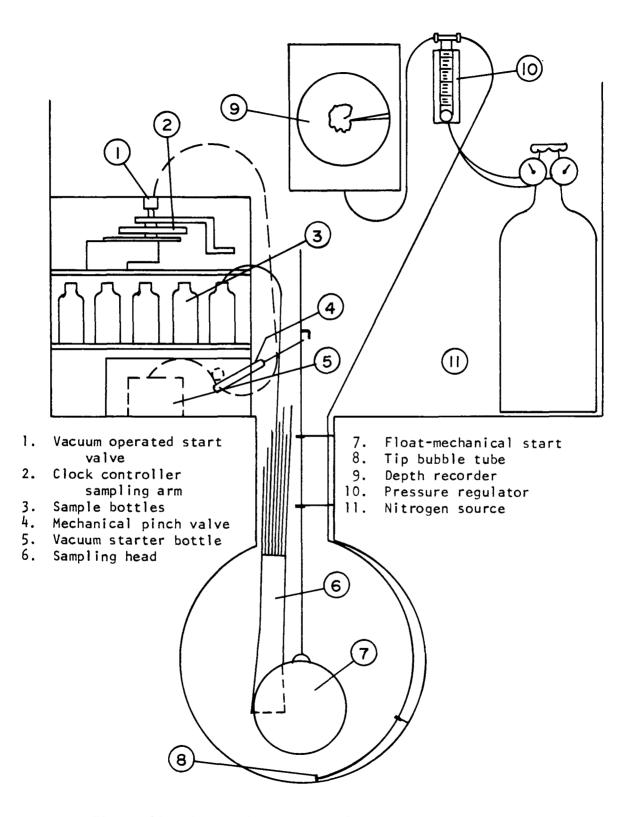
Figure 22. Schematic drawing of a typical monitoring site
