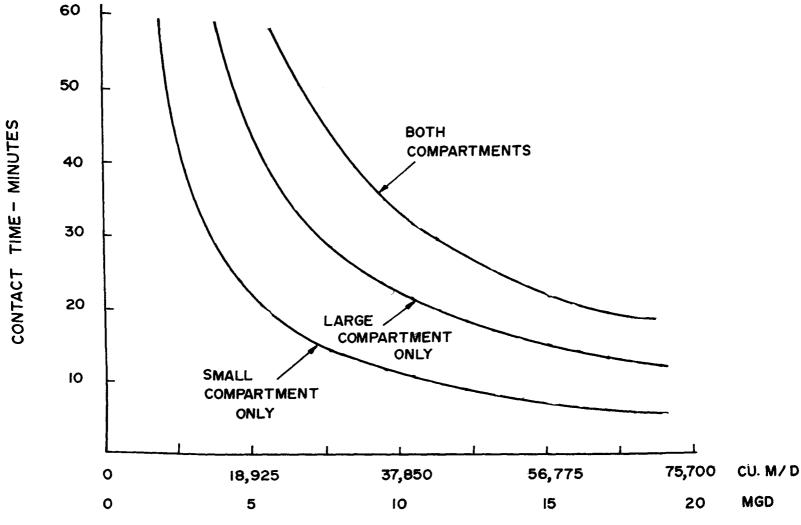
Figure 9. Contact times versus various flow rates
