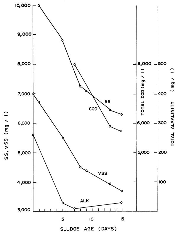
Figure 39. SS, VSS, Total COD, and Total Alkalinity Concentrations versus Sludge Age for Bench Scale Tests, August 8, 1973 to August 23, 1973
