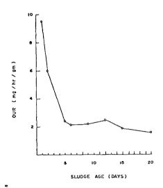
Figure 41. Oxygen Uptake Rate versus Sludge Age for Bench Scale Tests, July 11, 1973 to July 31, 1973
