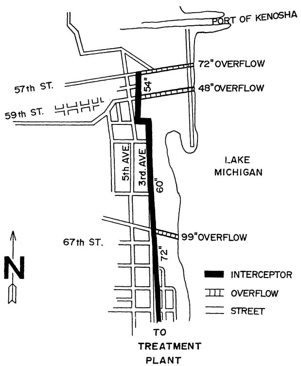
Figure 2. Illustration showing interceptor sewer and combined sewer overflow discharge locations
