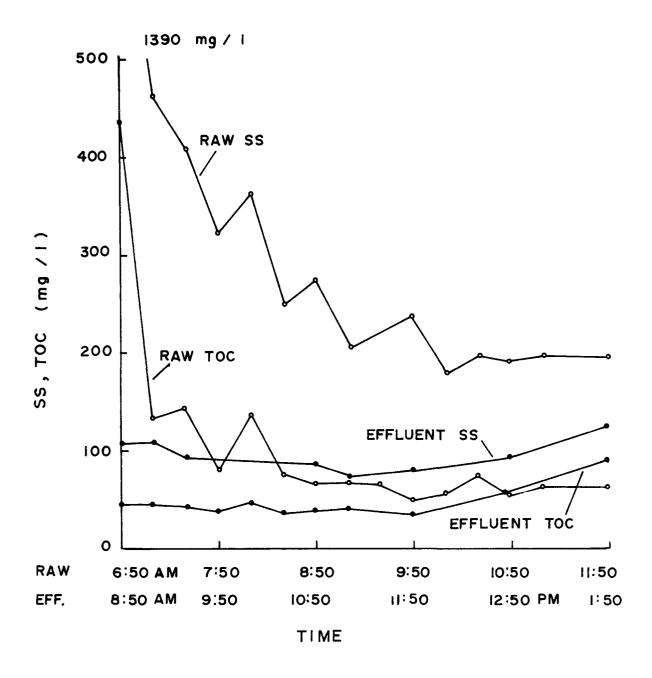
Figure 26. Raw and effluent sample quality variance through the dry weather plant primary sedimentation tanks during Run No. 47
