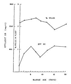
Figure 44. Flotation Test Percent Float Solids and Effluent SS versus Sludge Age for July 11, 1973 to July 31, 1973
