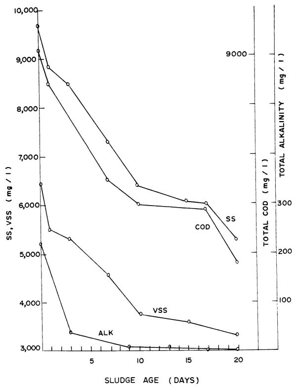
Figure 40. SS, VSS, Total COD, and Total Alkalinity Concentrations versus Sludge Age for Bench Scale Tests
