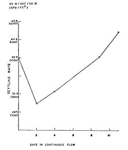
Figure 36. Calculated Surface Overflow Rate versus Days of Continuous Flow for July 9, 1973 to July 20, 1973
