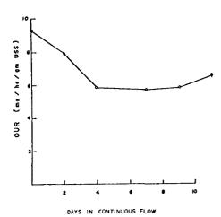
Figure 34. Oxygen Uptake Rate versus Days of Continuous Flow for July 9, 1973 to July 20, 1973
