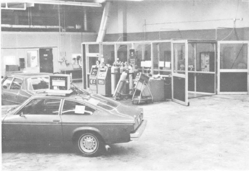
Figure 4-1 Evaporative Enclosure (front view).
