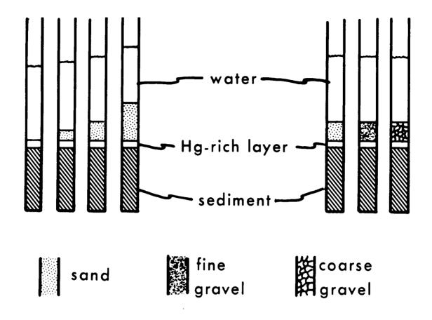
Figure 6. Schematic of laboratory incubation procedure.
