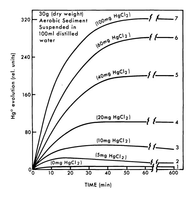
Figure 11. Rate of Hg<sup>O</sup> evolution from aerobic sediments spiked with HgCl<sub>2</sub>.
