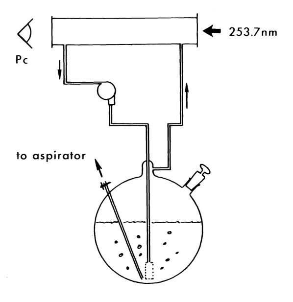
Figure 1. Schematic of closed system used for mercury analysis.
