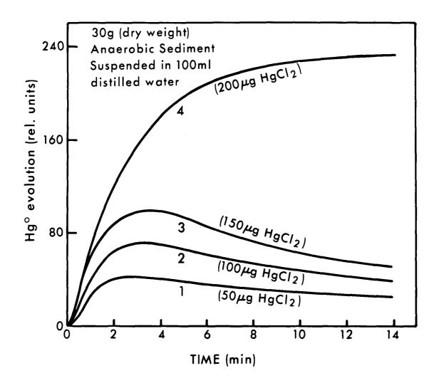
Figure 12. Rate of  ${\rm Hg}^{\rm O}$  evolution from anaerobic sediments spiked with 50  ${\rm \mu g}$  of  ${\rm HgCl}_2$ .
