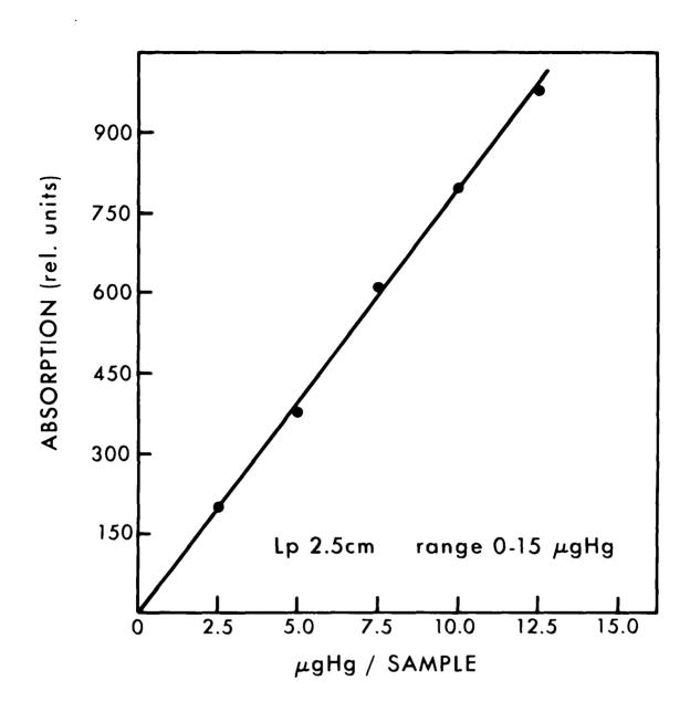
Figure 3. Calibration curve for absorption at 253.7 nm for mercury concentrations between 0 and 15 µg/sample.
