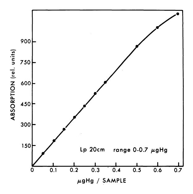
Figure 2. Calibration curve for absorption at 253.7 nm for mercury concentrations between 0 and 0.7 ug/sample.
