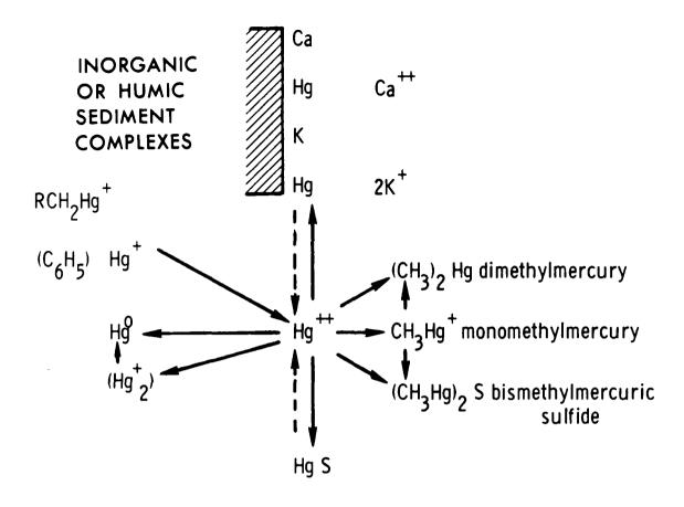
Figure 10. Transformation pathways of mercury and its derivatives in aquatic environment.
