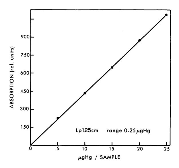
Figure 4. Calibration curve for absorption at 253.7 nm for mercury concentrations between 0 and 25 µg/sample.
