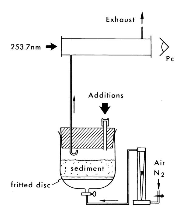
Figure 5. Schematic of flow-through system used to measure mercury vapor released directly from sediments.
