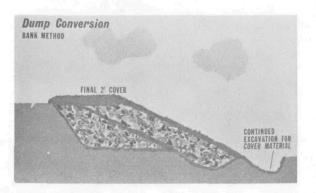
The bank method is a modification of the area method and merely takes advantage of the original sloping nature of the refuse. When the refuse has been set to a 3:1 slope, it is compacted and covered, thus forming the berms for the adjacent cell.
