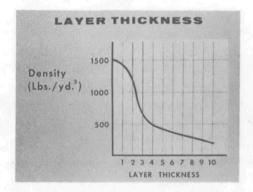
2 This recommended practice is based on field determinations which show that an optimum density is achieved by using a two foot thickness.
