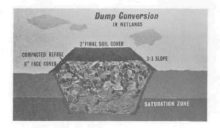
This method is used where the dump is in a marshland or in a river or other water course. The solid waste is first removed and then separated from the water by placement of a mat of impervious material that reaches above high water level.
