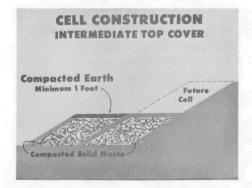
4 Building of cell continues (as outlined in step 1 above) until the day's incoming refuse is compacted in place or desired length is reached. The working face is then covered with 6" of compacted soil.
