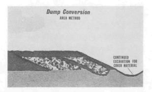
The area method is used where high water tables may prohibit the excavation of trenches.
