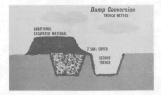
The trench method can be used where a high water table is not a problem.
