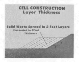
1 This technique requires the initial construction of a 3:1 slope or berm. Refuse is deposited at base of slope, spread upward in two foot layers and then compacted to about a one foot thickness.
