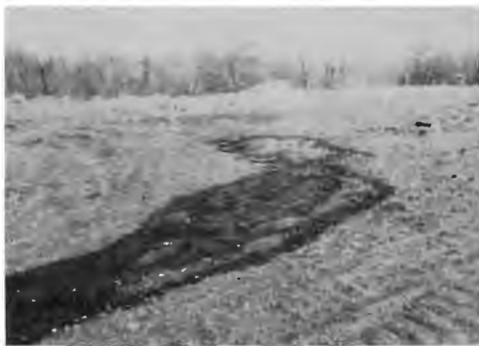
Figure 5 Contaminant Breakout Above Subsurface Tank No. 9
