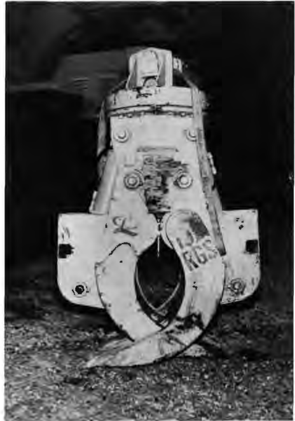
Figure 6 Grapple Used by Large Remotely Operated Vehicle for Grasping and Carrying Large Containers
