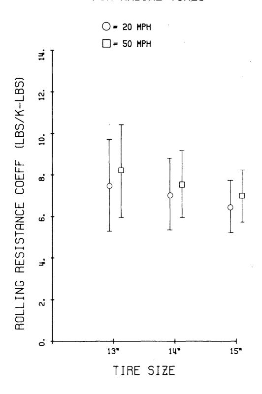
Fig. 5 - Means of the Radial Tire Rolling Resistance Coefficients by Tire Size. The error bars designate one standard deviation of the data.
