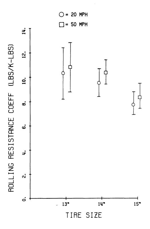
Fig. 6 - Means of the Bias Tire Rolling Resistance Coefficients by Tire Size. The error bars designate one standard deviation of the data.
