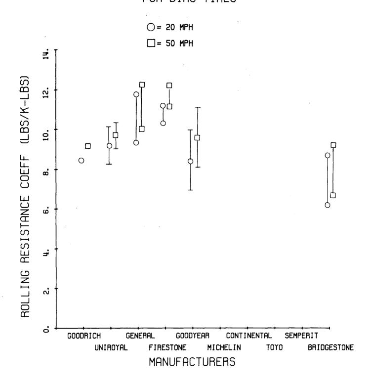
Fig. 4 - Means of the Bias Tire Rolling Resistance Coefficients by Manufacturer. The error bars designate one standard deviation of the data for those manufacturers where at least three observations occurred. If only one or two observations occurred, the plotted symbols designate the observed values.
