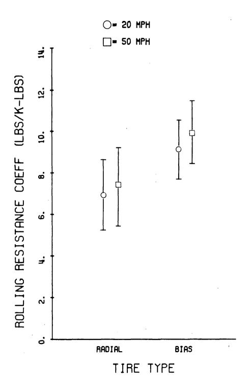
Fig. 2 - Means of the Tire Rolling Resistance Coefficients by Tire Type. The error bars designate one standard deviation of the data.
