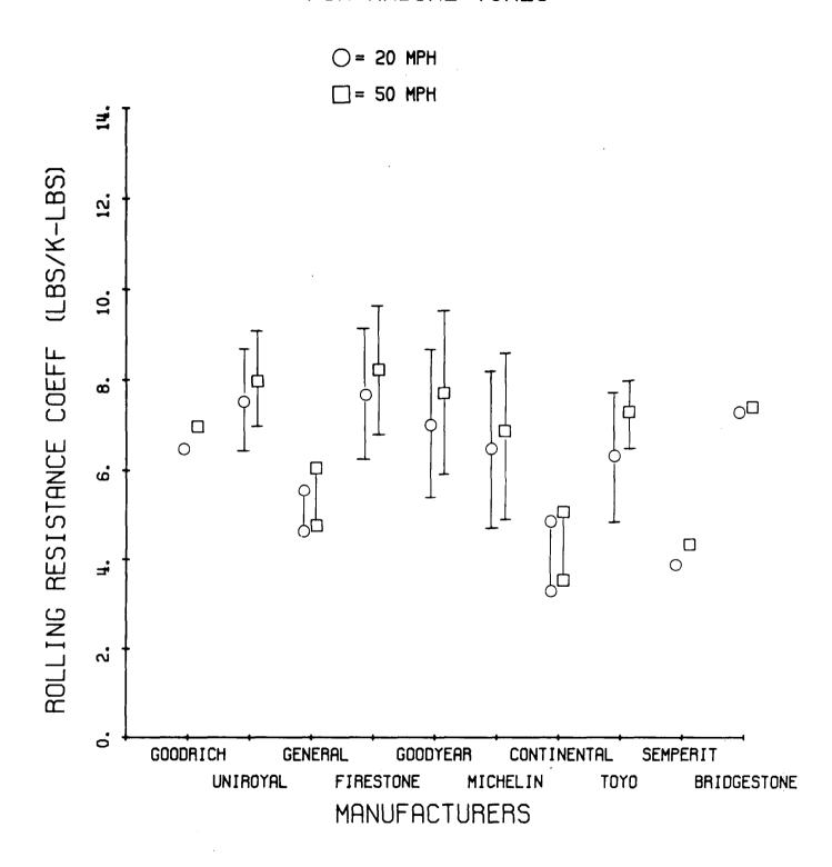
Fig 3. - Means of the Radial Tire Rolling Resistance Coefficients by Manufacturer. The error bars designate one standard deviation of the data for those manufacturers where at least three observations occurred. If only one or two observations occurred the plotted symbols designate the observed values.
