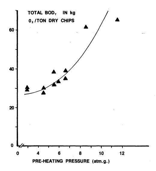
Figure V-1. Variation of BOD with pre-heating pressure
