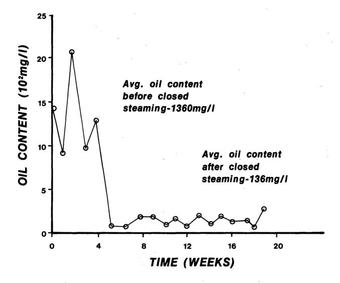
Figure VII-1 Variation in oil content of effluent with time before and after initiating closed steaming (Thompson and Dust, 1971)
