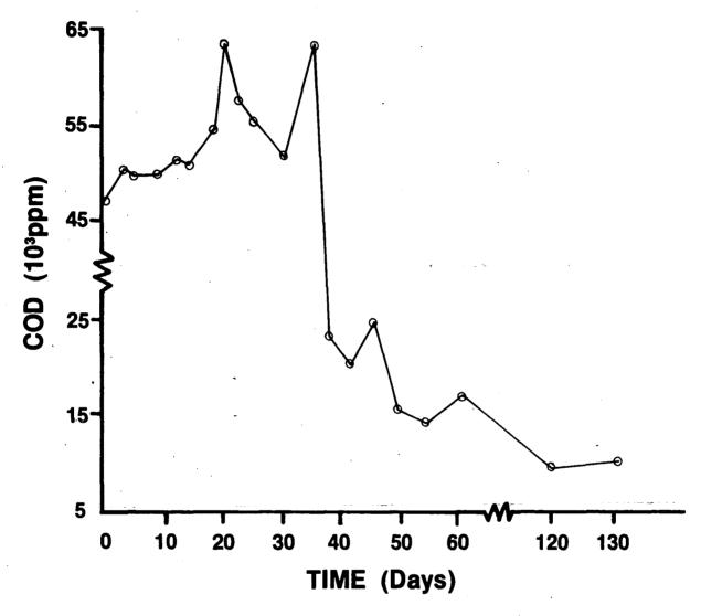
Figure VII - 2 Variation in COD of effluent with time before and after closed steaming: Days 0-35 open steaming; Days 35-130 closed steaming (Thompson and Dust,1971)
