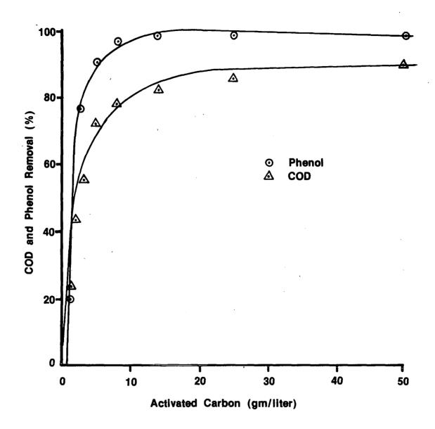
Relationship Between Weight of Activated Carbon Added and Removal of COD and Phenois from a Creosote Wastewater
