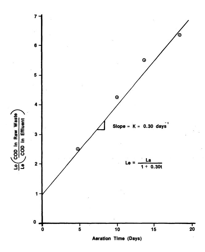
Determination of Reaction Rate Constant for a Creosote Wastewater
