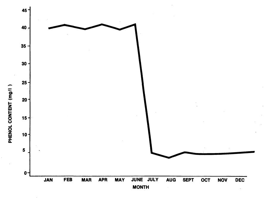
PHENOL CONTENT IN OXIDATION POND EFFLUENT BEFORE AND AFTER INSTALLATION IN JUNE 1966 OF AERATOR
