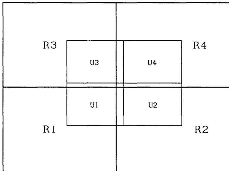
Figure N-4. Example set of ROM and UAM grid cells for the fractional area weighting method. (The ROM cells are about a factor of 4 larger than a UAM grid cell in this case.)
