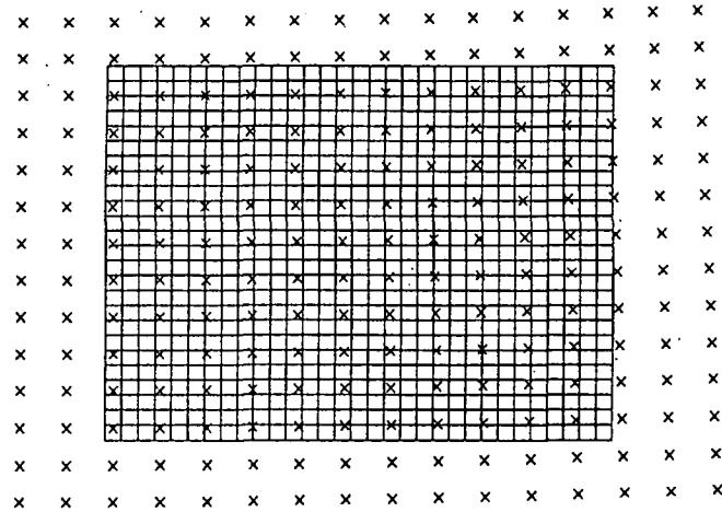
Figure N-1. Example of grid points (midpoints) of the ROM cells overlaying a UAM domain. Two ROM rows/columns extend beyond each UAM boundary.
