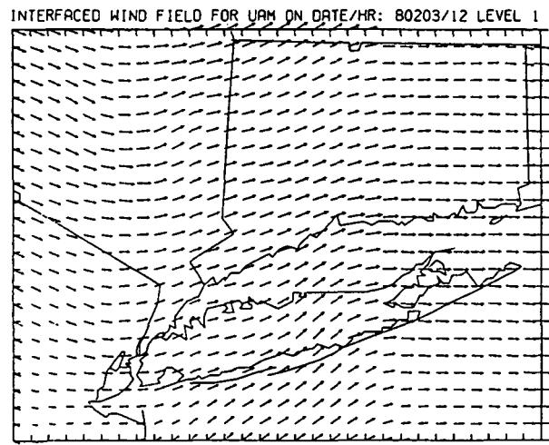
Figure N-3. Wind field derived for an example UAM grid from the ROM gridded wind components.
