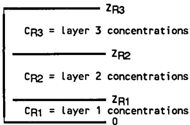
**Example Configuration of UAM Vertical Levels (thicknesses not to scale):**
