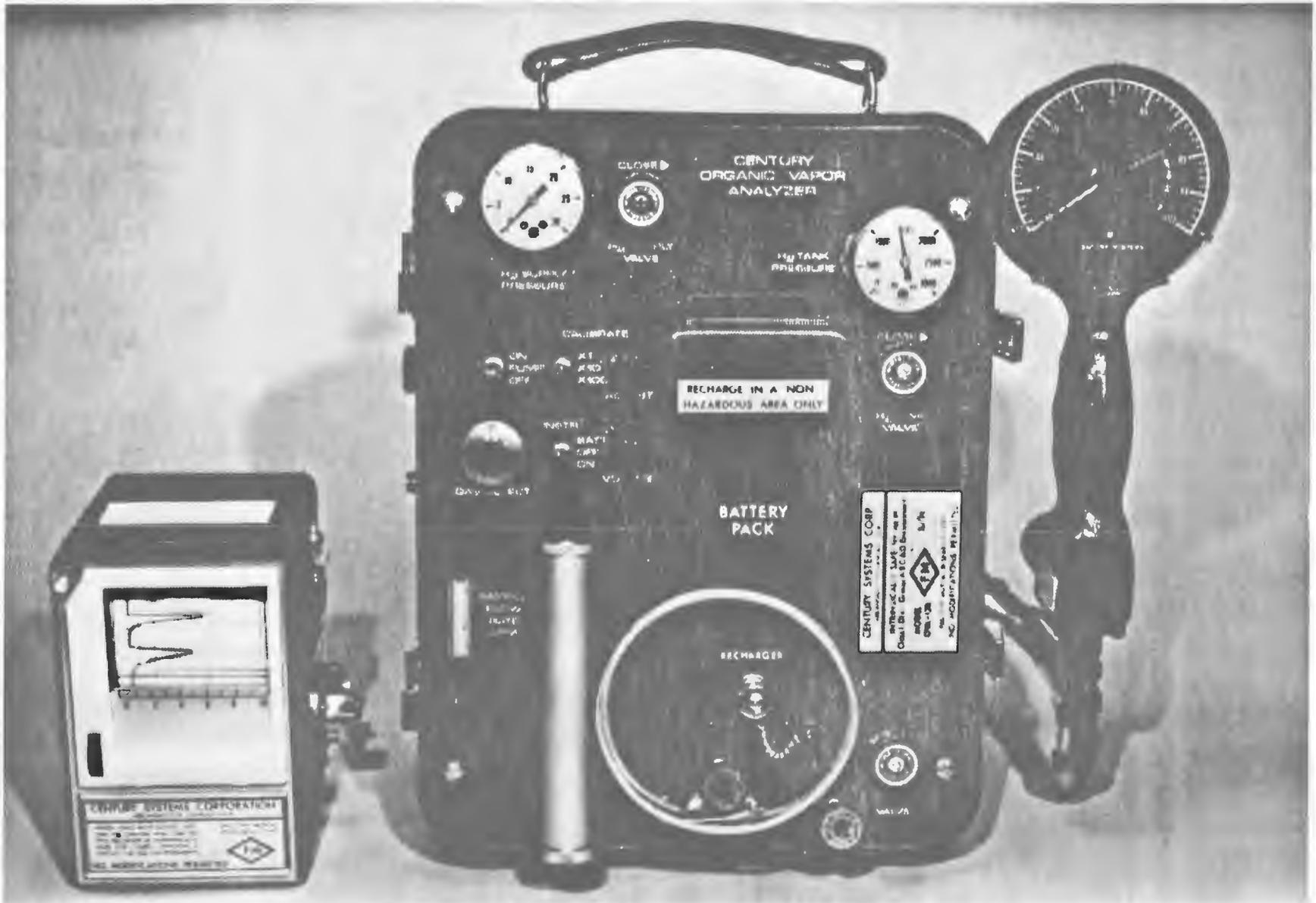
Figure G-1. Portable organic vapor analyzer (Model OVA-128).
