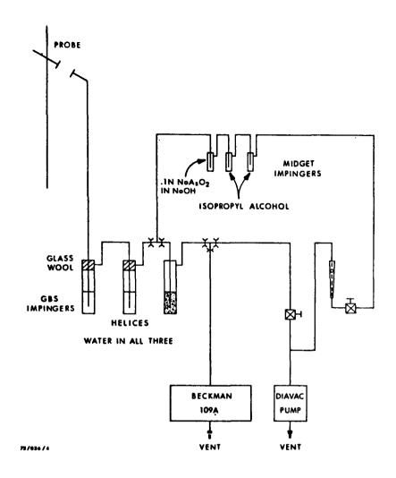
Figure V-1. Sampling Train for Stack Gas Analysis, Research Burn I
