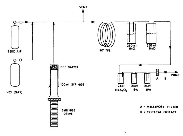
Figure 15. Laboratory Apparatus for Sample Recovery - Integrity Test
