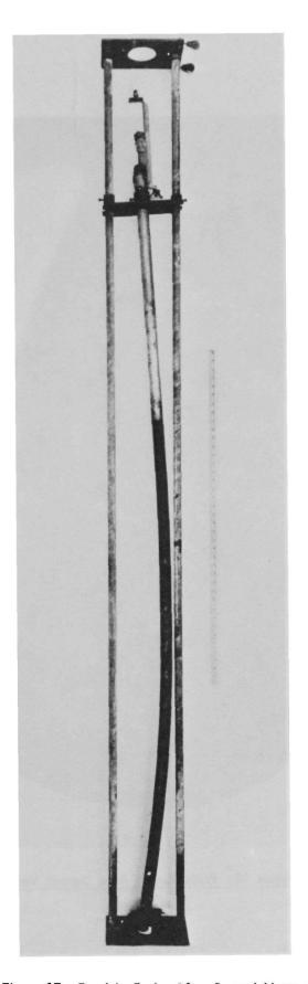
Figure 17. Bend in Probe After Second Voyage
