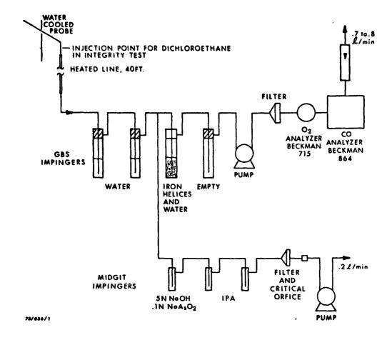
Figure V-2. Sampling Train for Stack Gas Analysis, Research Burn II
