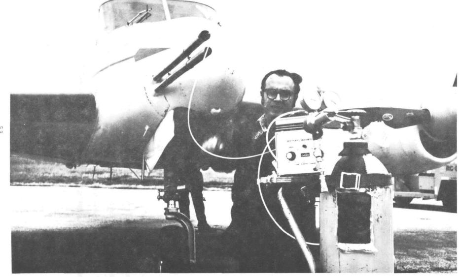
Figure V-3 Environmental Protection Agency NERC — Las Vegas aircraft with sampling probes and monitoring instruments.
