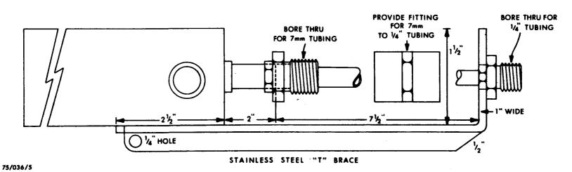
Figure 9. Probe Dimensions — Second Voyage
