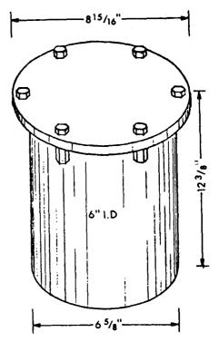
PRESSURE VESSEL FOR USE IN GRAVITY CONVECTION OVEN.
