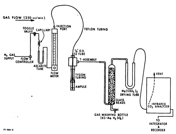
Figure 2. Flow Diagram of the Equipment Used for Determining the Carbon Dioxide Generated by the Wet Oxidation of Organic Matter in Water
