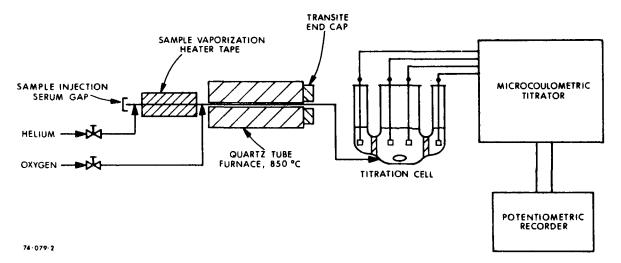
Combustion - Coulometric Apparatus for the Determination of Organic Chlorides Figure 3.
