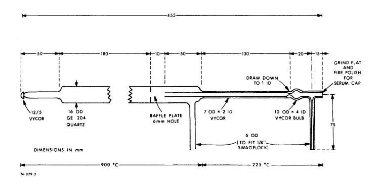
Figure 1. Quartz Tube for the Vaporization and Combustion of Trace Amounts of Organic Chlorides
