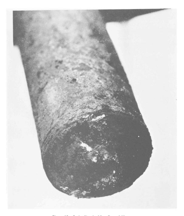
Figure 18. Probe Nozzle After Second Voyage
