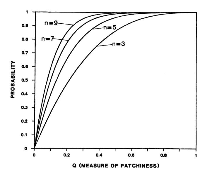
Figure 1. Probability of finding asbestos when it is present as a function of Q (where Q is the probability that asbestos is in the sample when the surfacing material in the homogenous sampling area contains at least (1% asbestos) for sample sizes of 3, 5, 7, and 9.
