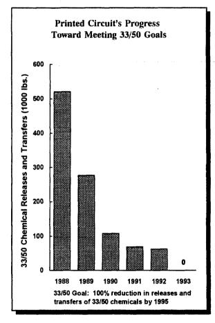
As a result of the study, the company has replaced its use of 1,1,1-trichloroethane as a developing agent with a water-based sodium carbonate solution. In addition, Printed Circuit now uses a mild detergent with water for the final cleaning of completed circuit boards, in place of dichloromethane and 1,1,1-trichloroethane.
