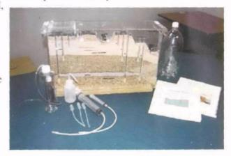
enables audiences to understand and visualize in color, the nature, behavior, and contamination of groundwater, an otherwise invisible and often unimaginable natural resource. Different color dyes injected into the various, common routes to groundwater show patterns that help illustrate these principles. Pumping water
