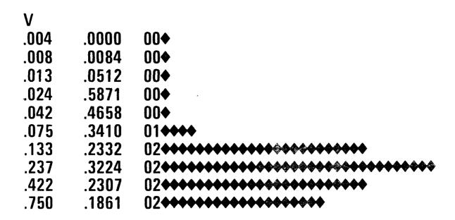
Figure 2. Result of an ambient indoor aerosol measurement, illustrating tabular and histogram outputs. The first column lists the average particle diameter (in  $\mu$ m), while the second and third columns give the corresponding volume distribution values  $\Delta V/\Delta logD$  (in  $\mu$ m) as a fraction and power of 10, respectively.
