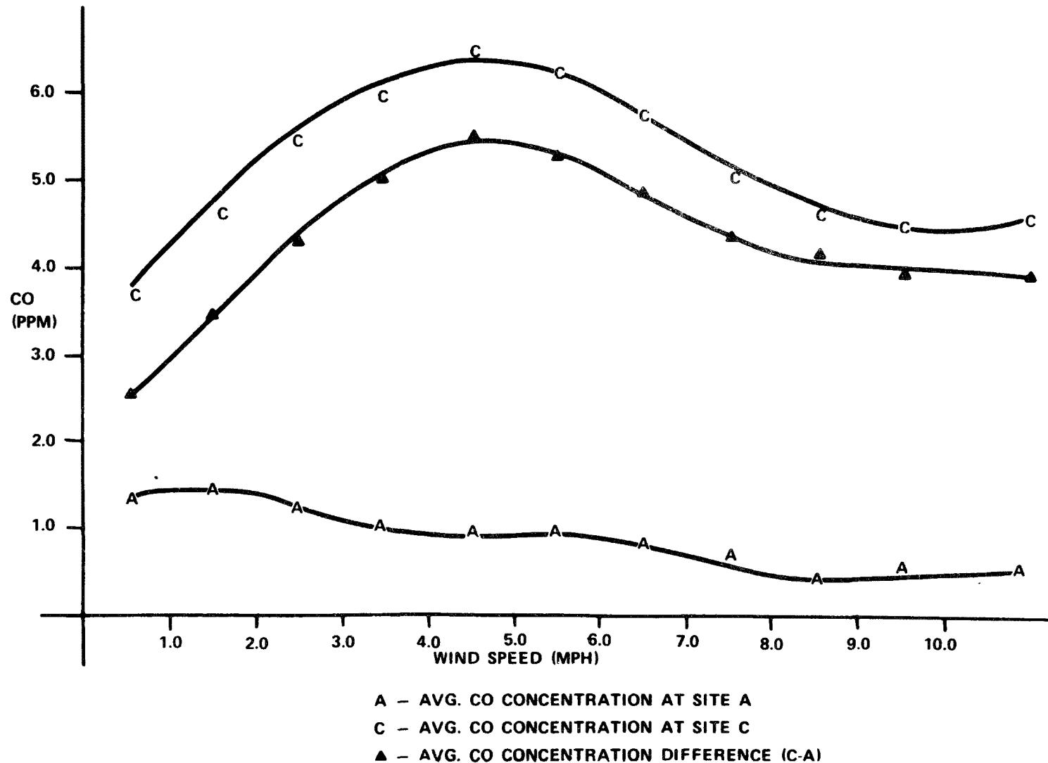
Figure 10. CO by wind speed for WD=SW.
