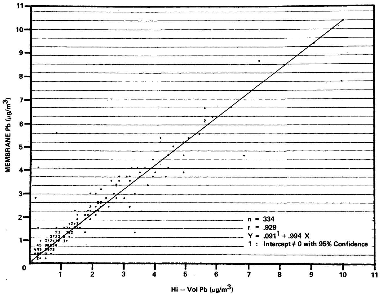
Figure 53. Membrane Pb vs. Hi-Vol Pb. Site A: 1500-1800 hours.
