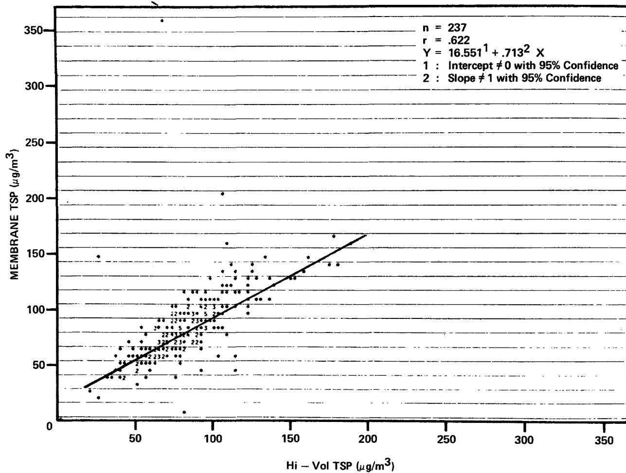
Figure 51. Membrane TSP vs. Hi-Vol TSP. Site B: 0-2300 hours.
