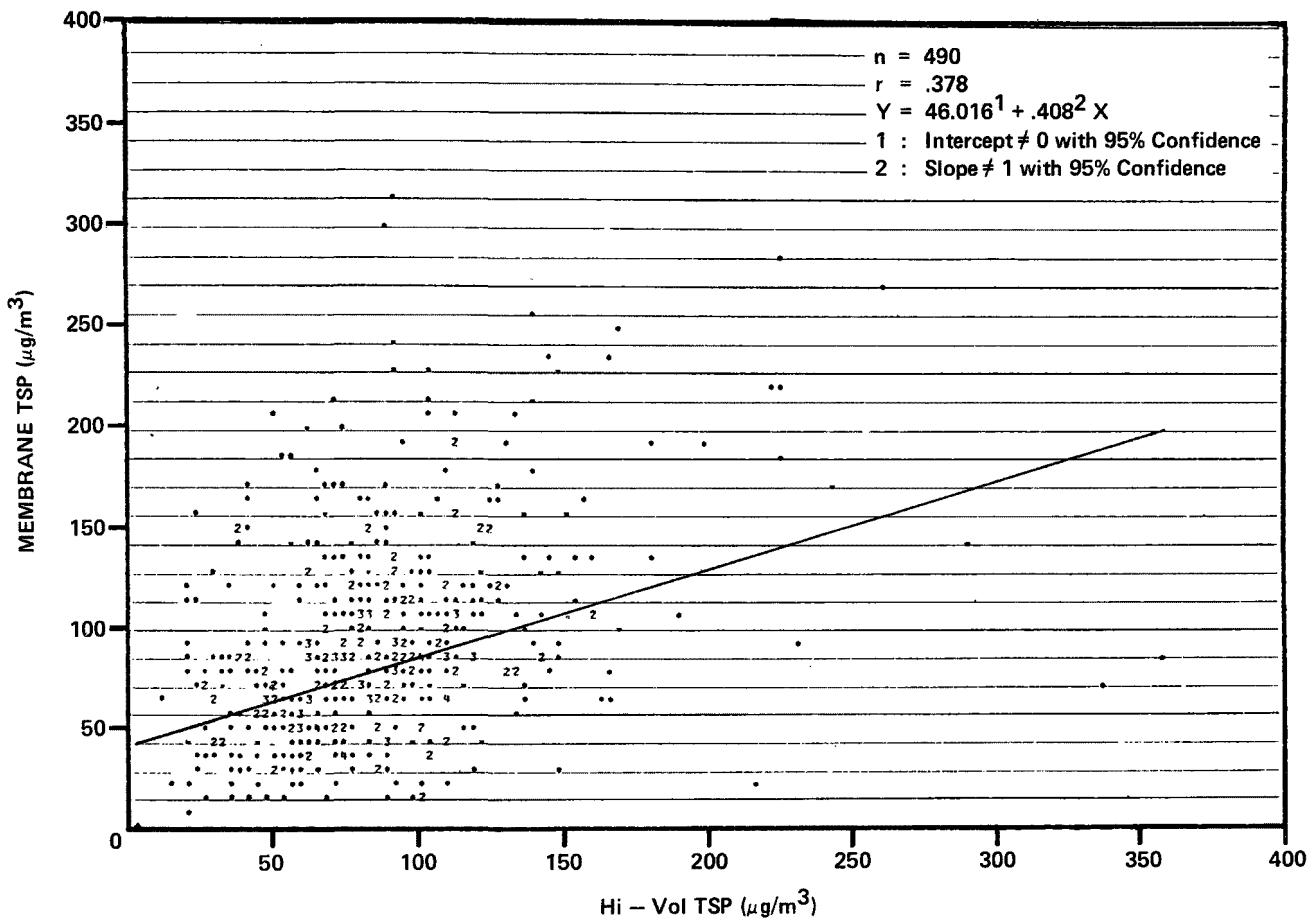
Figure 49. Membrane TSP vs. Hi-Vol TSP. Site A: 1500-1800 hours.
