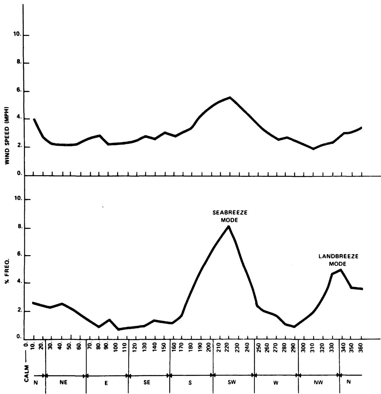
Figure 4. Percent frequency and speed by wind direction (all data).
