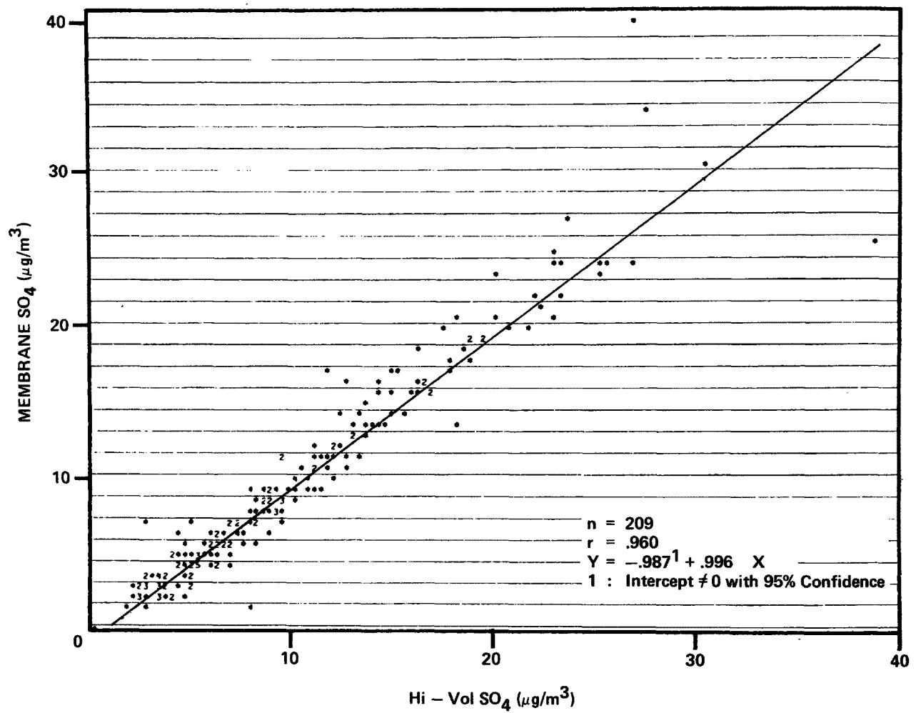
Figure 59. Membrane  $\text{SO}_4$  vs. Hi-Vol  $\text{SO}_4$ . Site B: 0-2300 hours.
