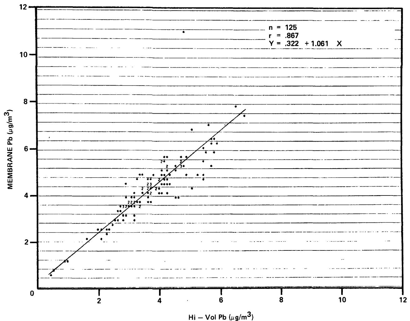
Figure 56. Membrane Pb vs. Hi-Vol Pb. Site D: 0-2300 hours.
