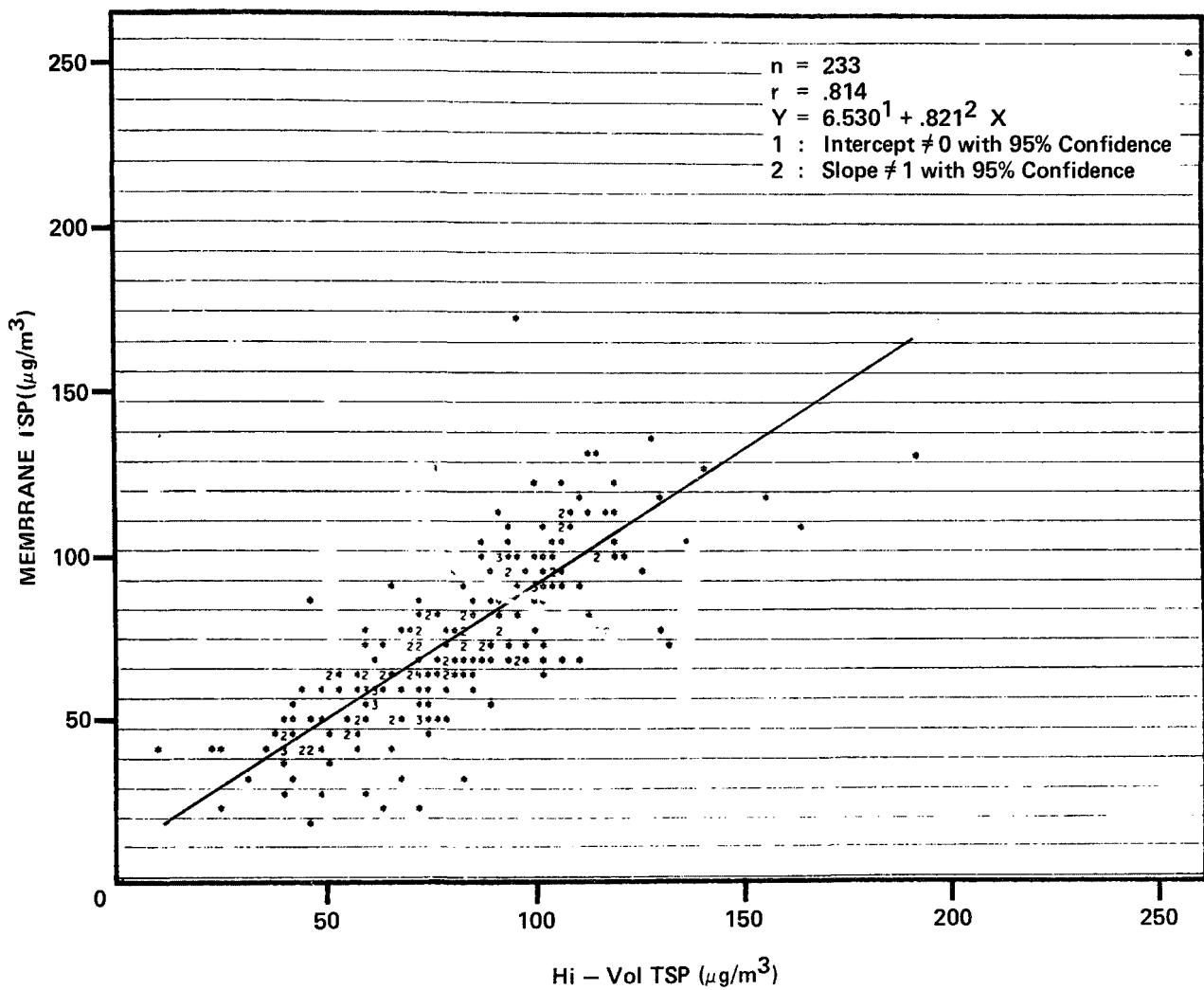
Figure 52. Membrane TSP vs. Hi-Vol TSP. Site D: 0-2300 hours.
