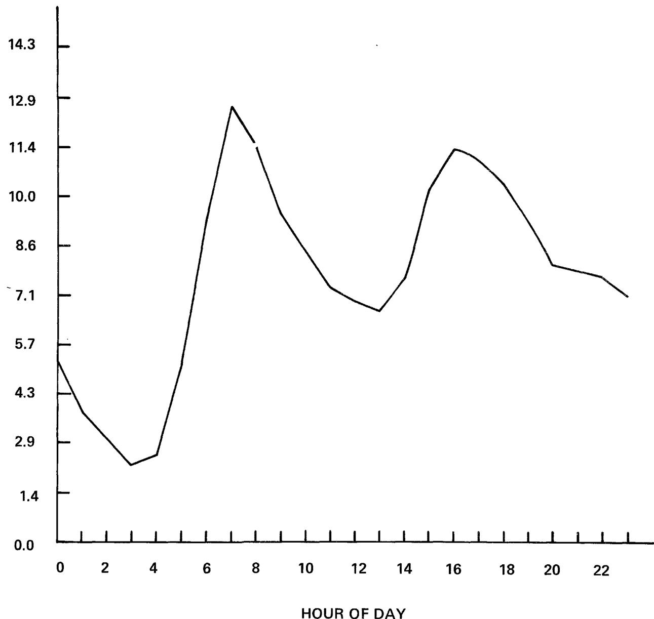
Figure 27. Carbon monoxide by hour (freeway median).
