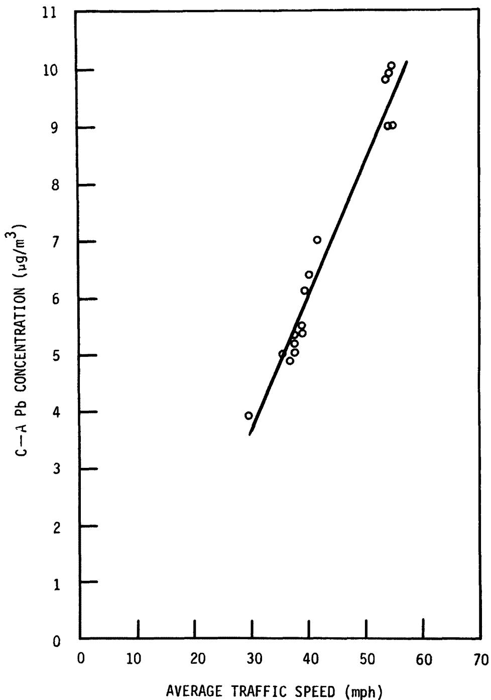
Figure 28.  $\Delta(\text{C}-\text{A})$  Pb concentrations vs. average traffic speed.
