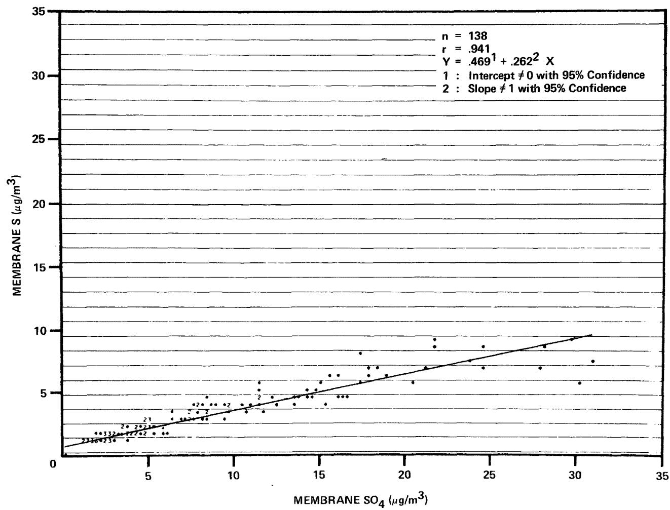
Figure 64. Membrane S vs. Membrane  $\text{SO}_4$ . Site D: 0-2300 hours.
