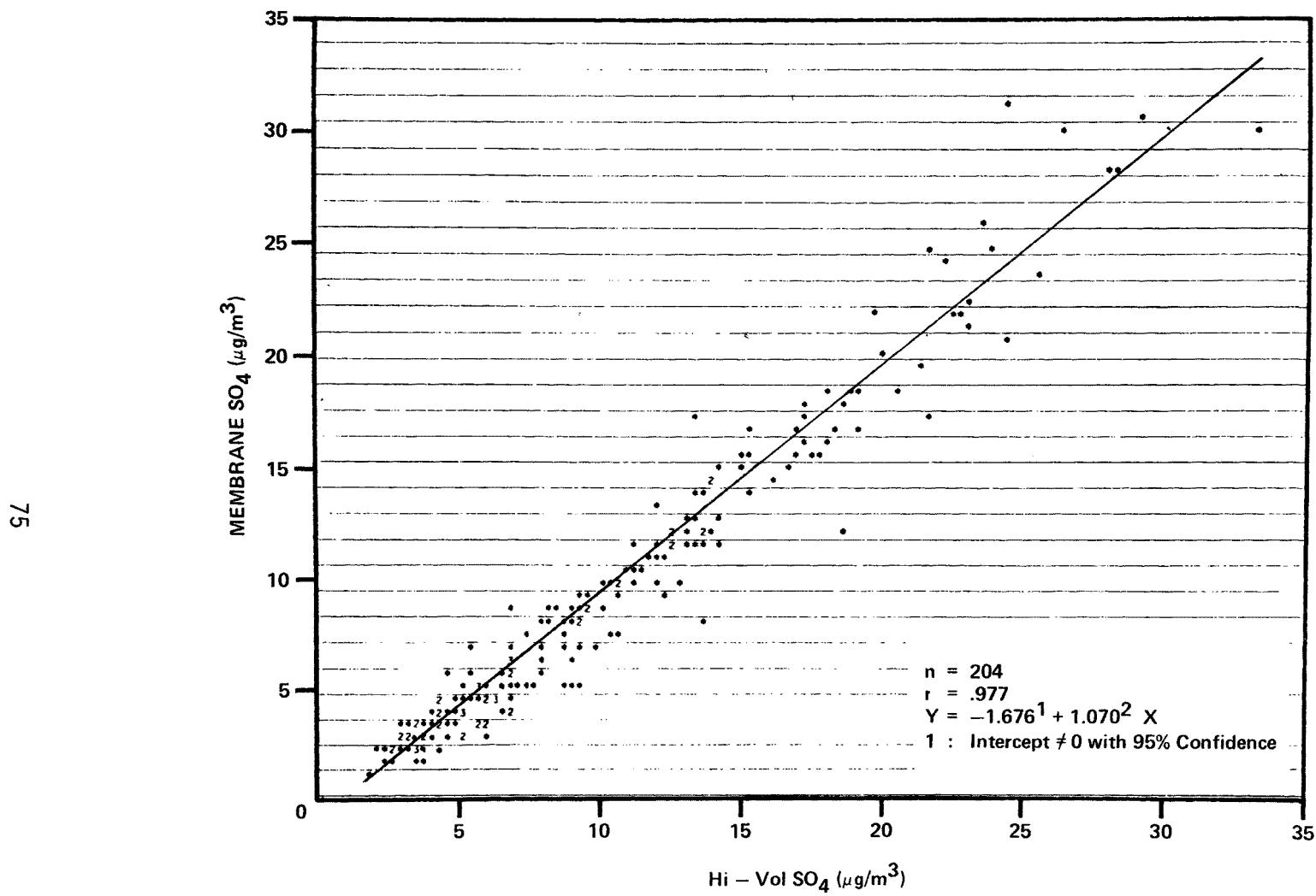
Figure 60. Membrane  $\text{SO}_4$  vs. Hi-Vol  $\text{SO}_4$ . Site D: 0-2300 hours.
