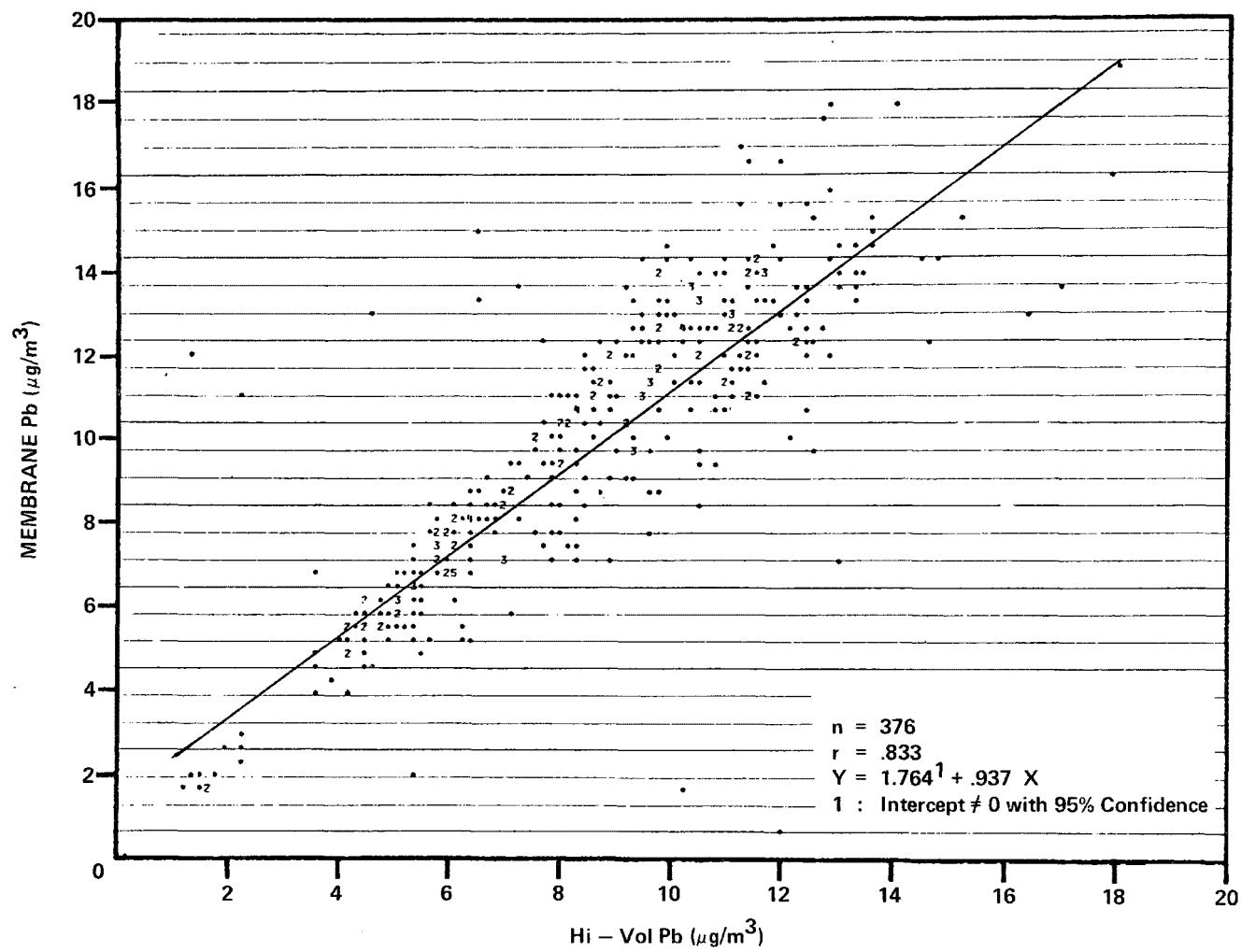
Figure 54. Membrane Pb vs. Hi-Vol Pb. Site C: 1500-1800 hours.
