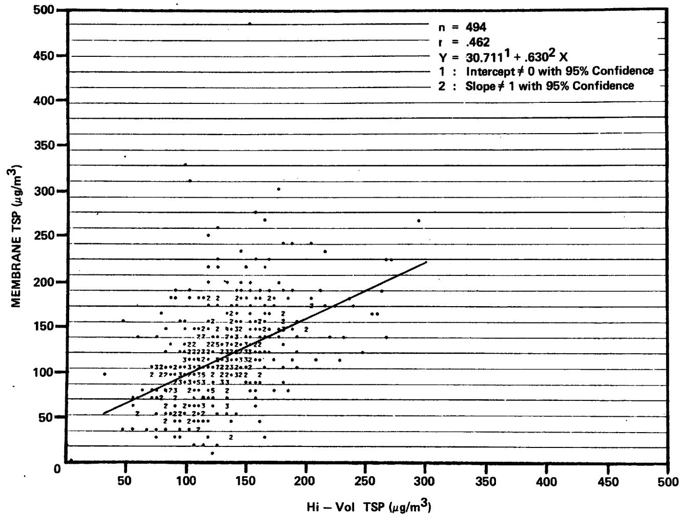
Figure 50. Membrane TSP vs. Hi-Vol TSP. Site C: 1500-1800 hours.
