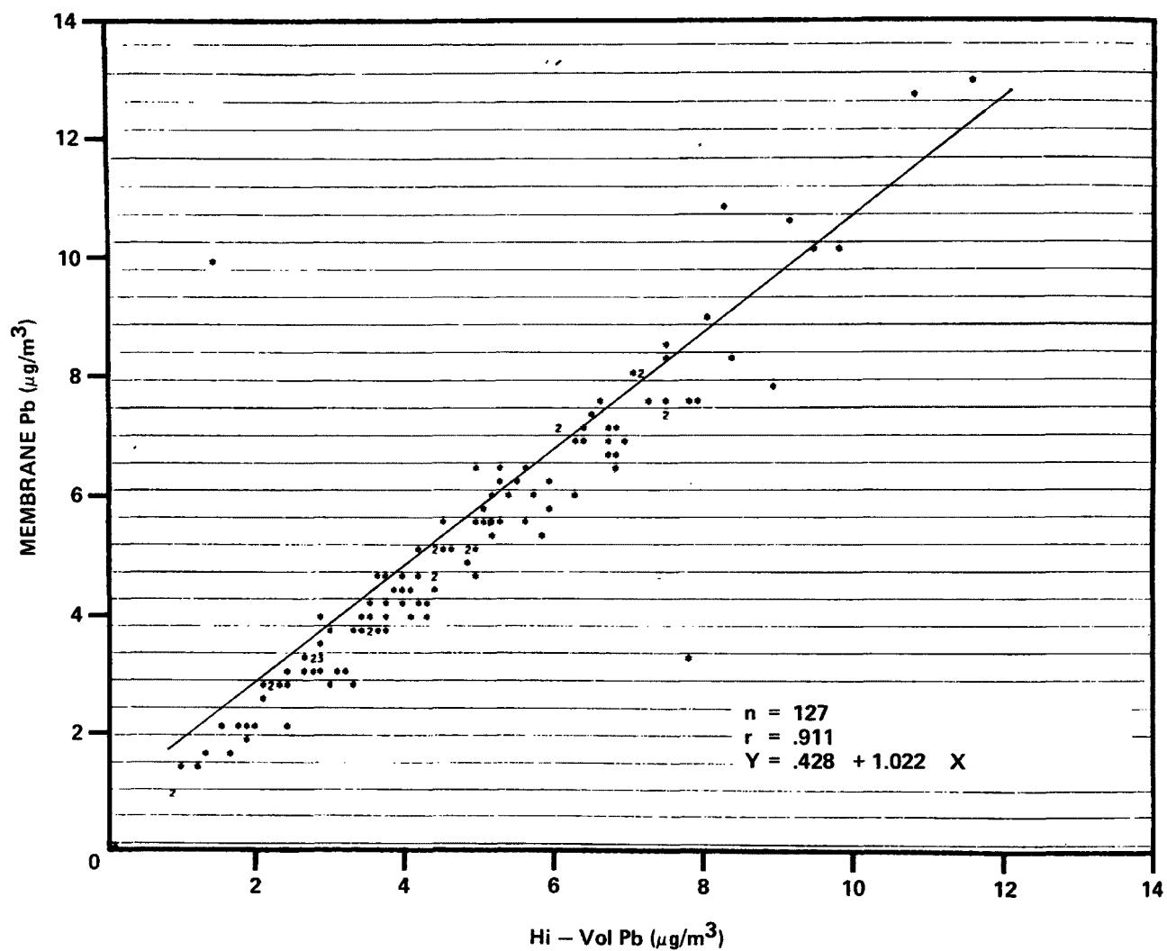
Figure 55. Membrane Pb vs. Hi-Vol Pb. Site B: 0-2300 hours.
