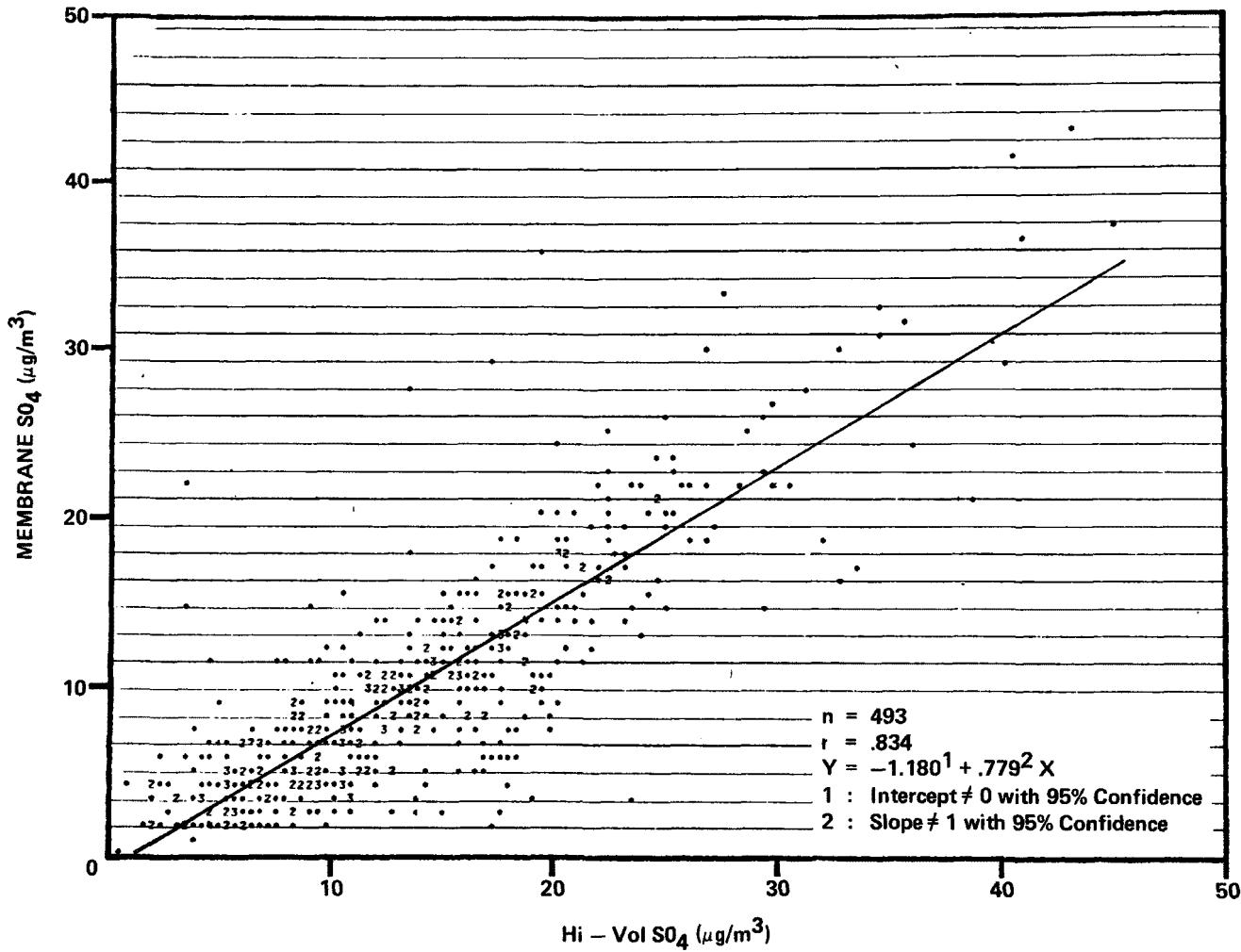
Figure 57. Membrane SO<sub>4</sub> vs. Hi-Vol SO<sub>4</sub>. Site A: 1500-1800 hours.
