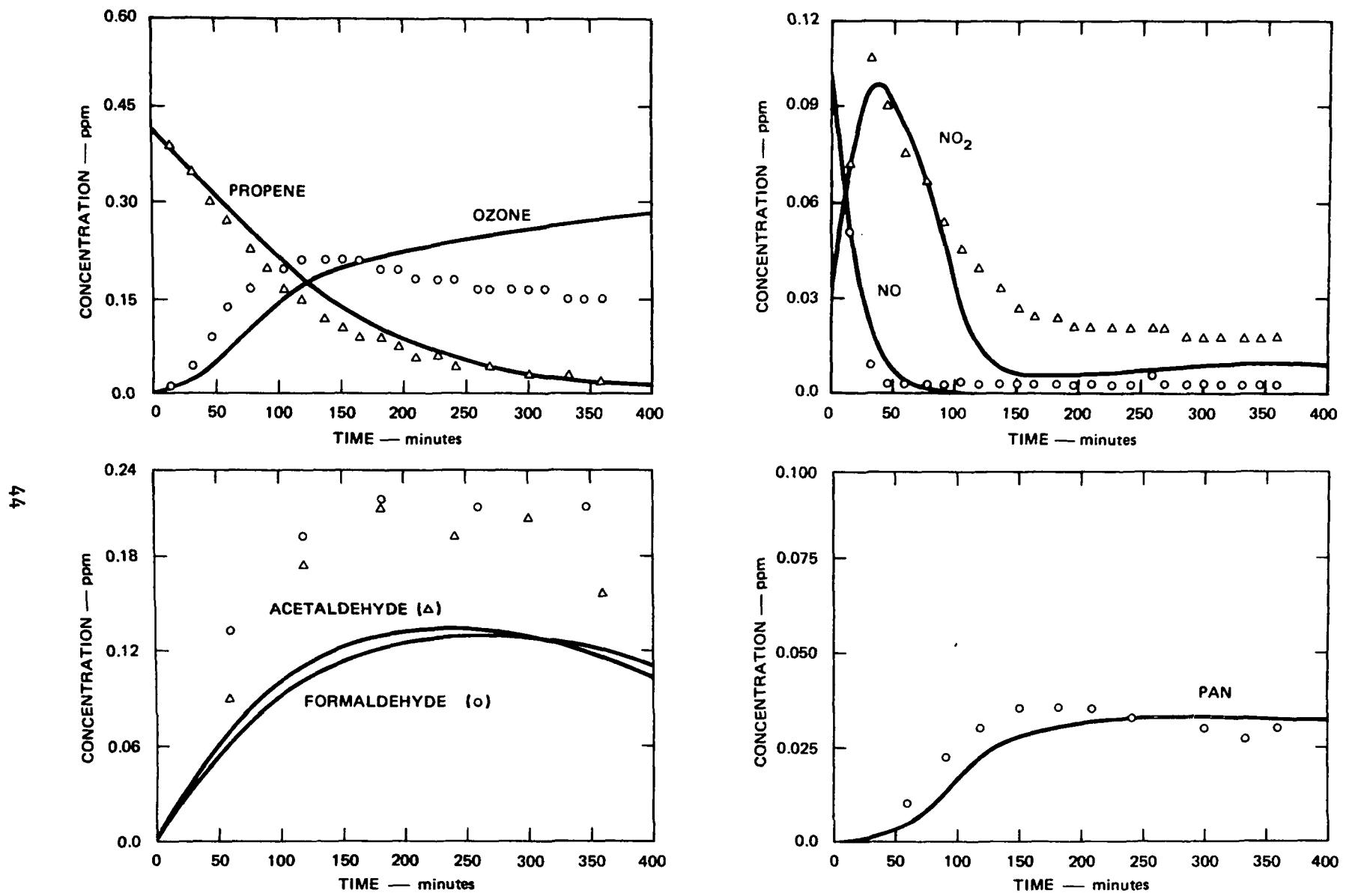
Figure 7. Simulation of SAPRC EC-11: 0.447 ppm Propene and 0.135 ppm NO<sub>x</sub>.
