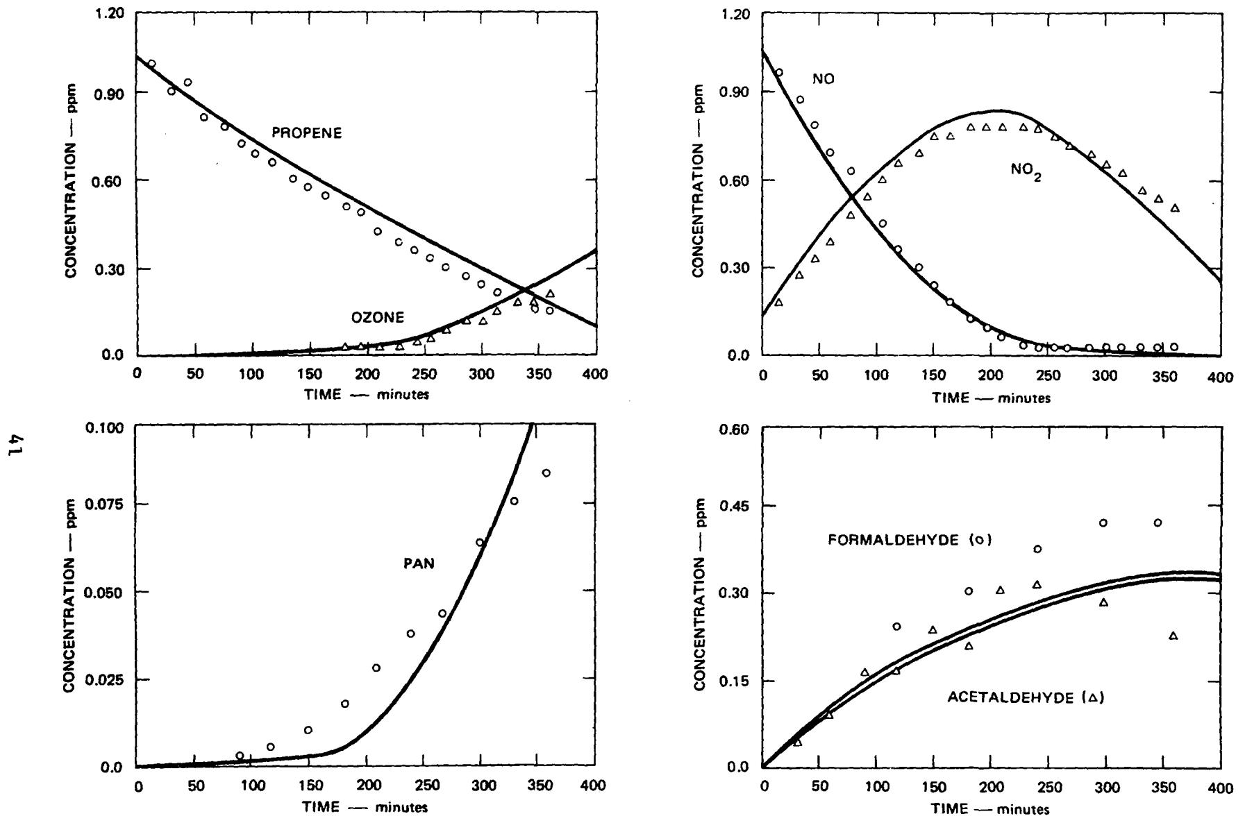
Figure 4. Simulation of SAPRC EC-60: 1.04 ppm Propene and 1.25 ppm NO<sub>x</sub>.
