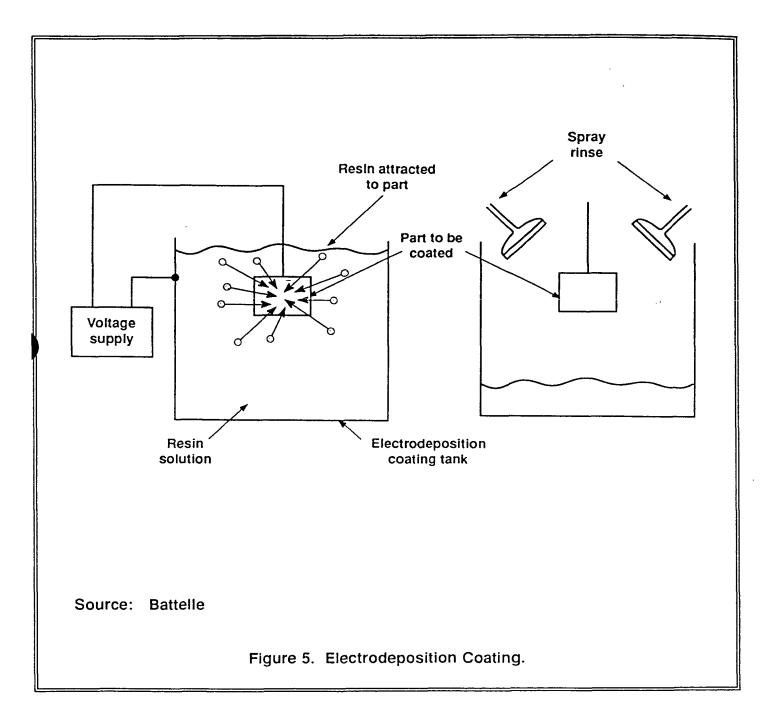
The electrodeposition technology does, however, require special equipment and procedures resulting in high installation and other costs. Electrodeposition requires new coating tanks, extra-clean
