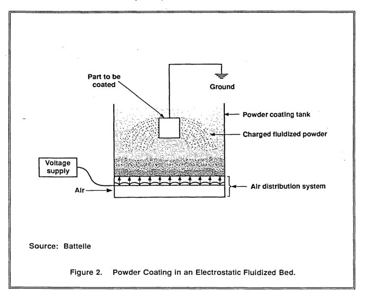
In electrostatic applications, the dry powder is applied to the unheated substrate as film of powder held in place by electrostatic forces. The substrate or a primer coat must be electrically conductive. The substrate, with powder coating, is then heated in an oven to melt and cure the coating. Additional polymerization and cross-linking occurs in the thermoplastic material during curing.
