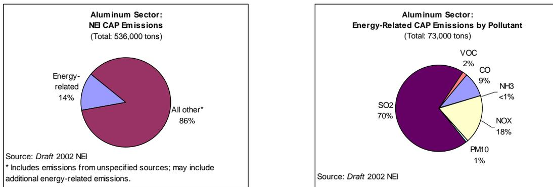
Figure 6 compares NEI data on energy-related CAP emissions with non-energy-related CAP emissions for the aluminum sector. According to the figure, energy-related CAP emissions are a relatively small fraction of total emissions; however, NEI data attribute emissions from the generation of purchased energy to the generating source, not the purchasing entity. Therefore,
