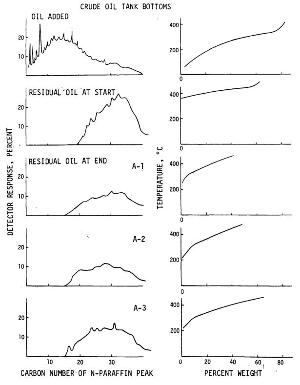
GAS CHROMATOGRAPH AND BOILING POINT PROFILES, "A" PLOTS
