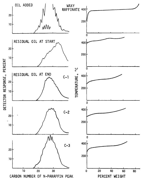
GAS CHROMATOGRAPH AND BOILING POINT PROFILES, "C" PLOTS
