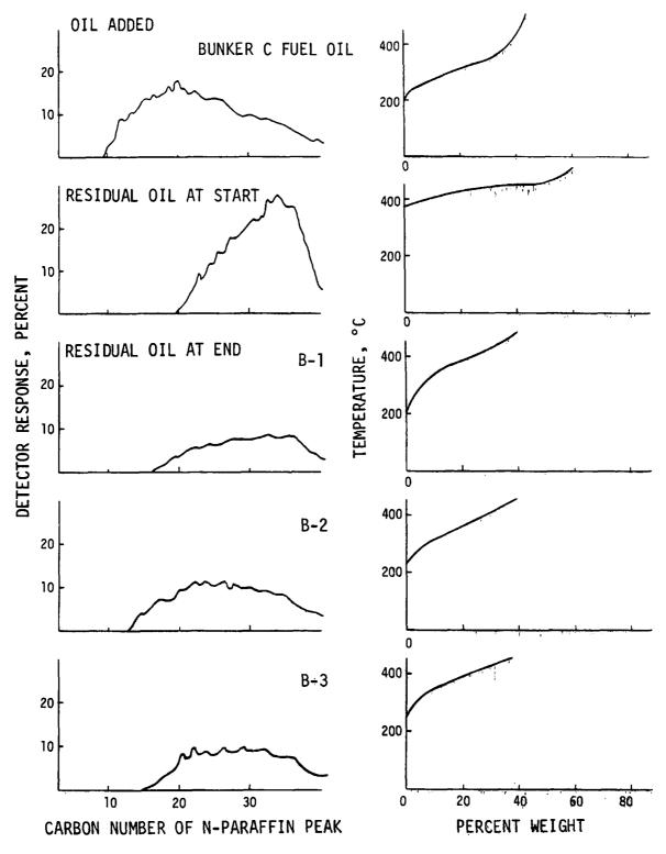
GAS CHROMATOGRAPH AND BOILING POINT PROFILES, "B" PLOTS
