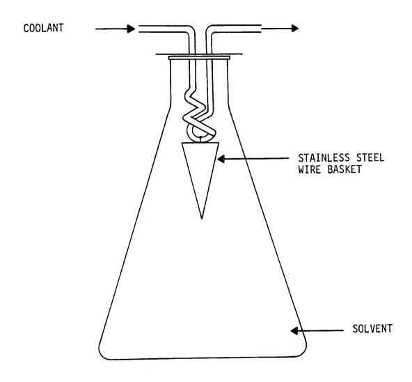
APPARATUS FOR EXTRACTION OF OIL IN SOIL
