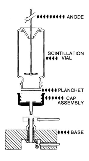
Figure 1. Disposable electrodeposition cell and support
