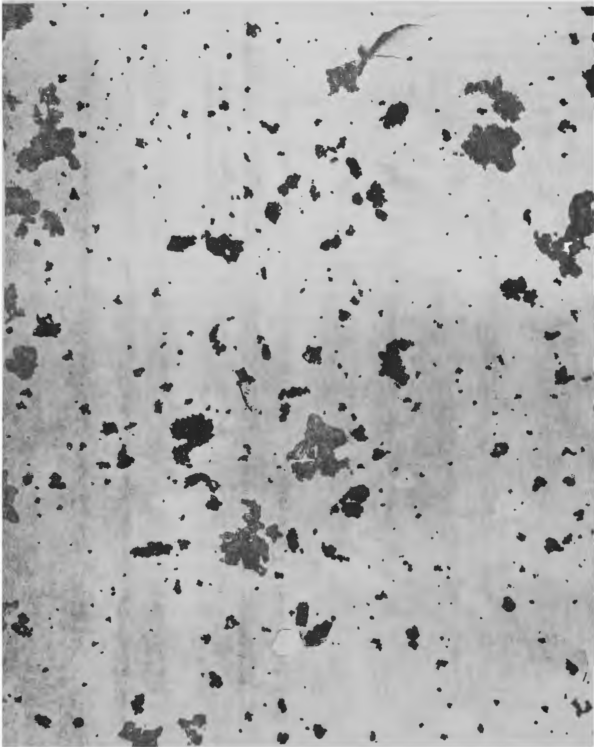
Figure 17.9. Photomicrograph of Emissions from Sinter Plants, 7800X, After Mechanical Collector.
