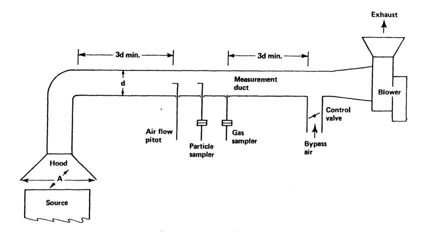
"Figure 2. Typical Survey Sampling System."
