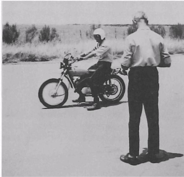
Figure 21. Idle Noise Being Measured from the Left Side of the Kawasaki 125F-6 Motorcycle
