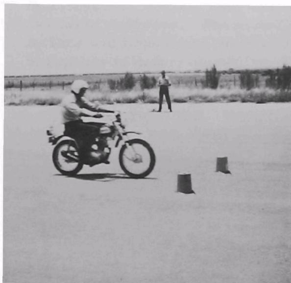
**Figure 18.** Noise Measurement on Honda SL100 Motorcycle From Side 1 During Right-to-Left Acceleration Run
