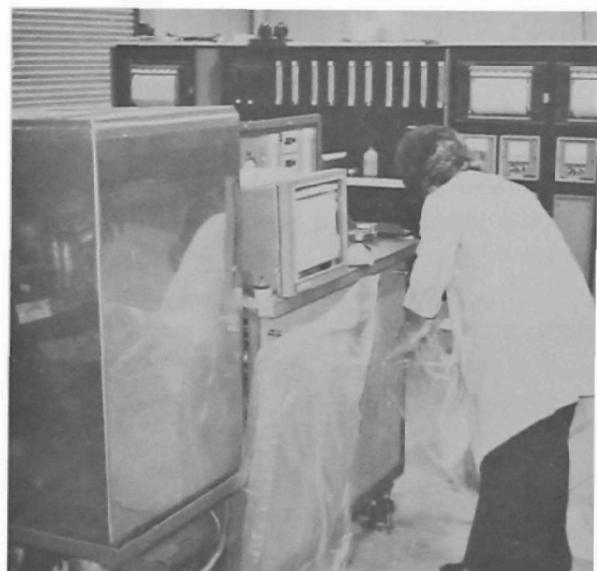
Figure 7. Technician Removing Dilute Sample Bags from Constant Volume Sampler
