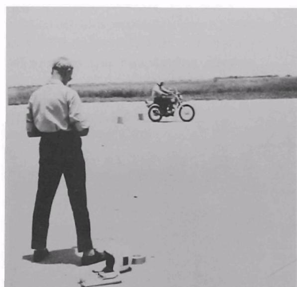
**Figure 19.** Noise Measurement on Honda SL100 Motorcycle from Side 1 During Left-to-Right Acceleration Run
