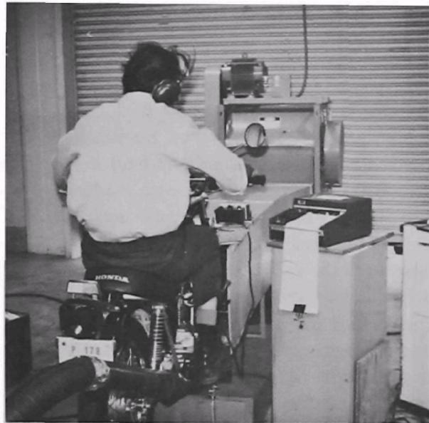
Figure 4. Motorcycle Operator Following Strip Chart Driving Aid During Emission Test
