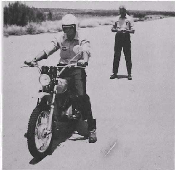
Figure 20. Idle Noise Being Measured from the Rear of the Kawasaki 125F-6 Motorcycle
