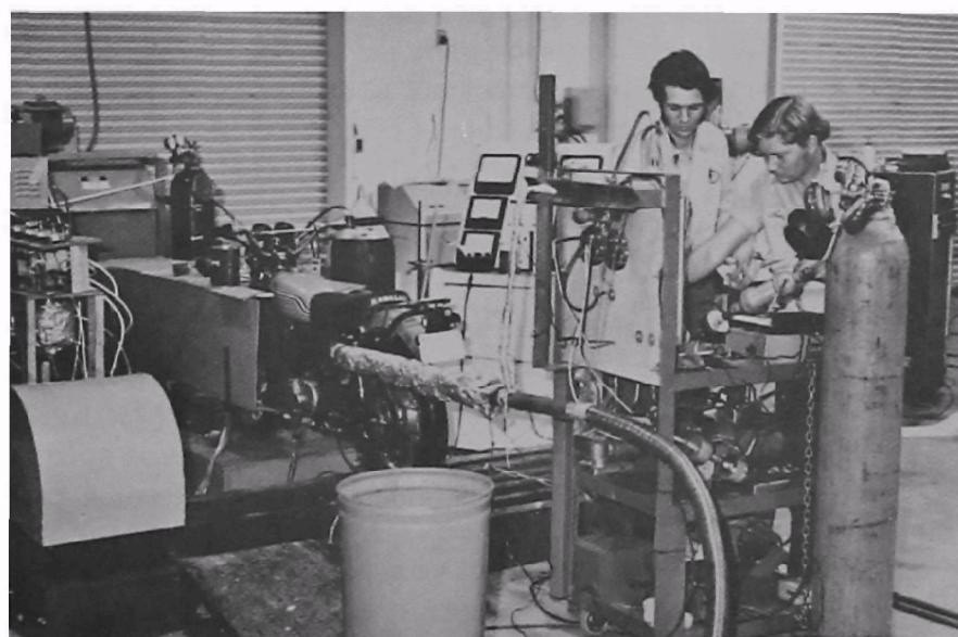
Figure 13. Rear View of Particulate Sampler
