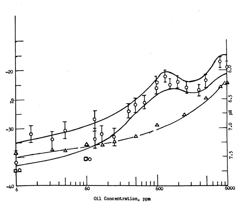
A spent "A" rolling oil emulsion was also examined. After filtration over a 0.8 micrometer Millipore filter pad a 3,100 ppm emulsion was obtained. The zeta potential of the system was approximately -24 mv. Dilution with mill mix water in binary steps to 39 ppm failed to produce any significant change in zeta potential.
