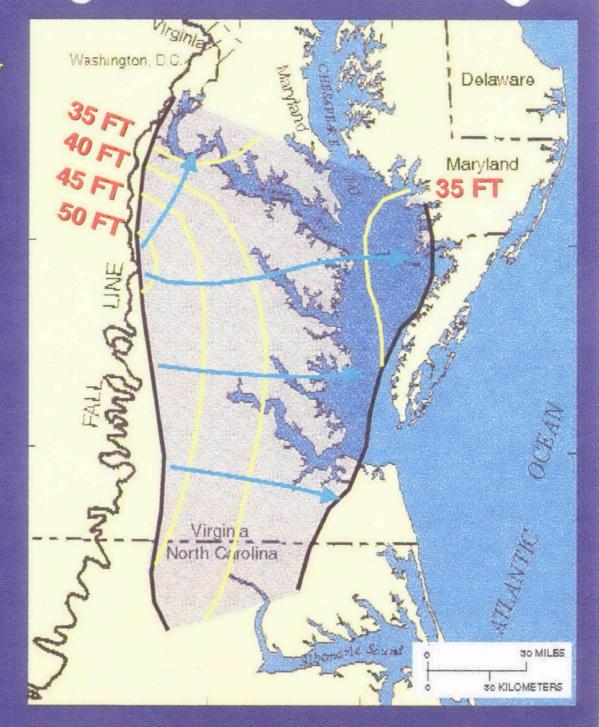
Measured Modern (1990's) Water Levels in the Lower Potomac Aquifer
