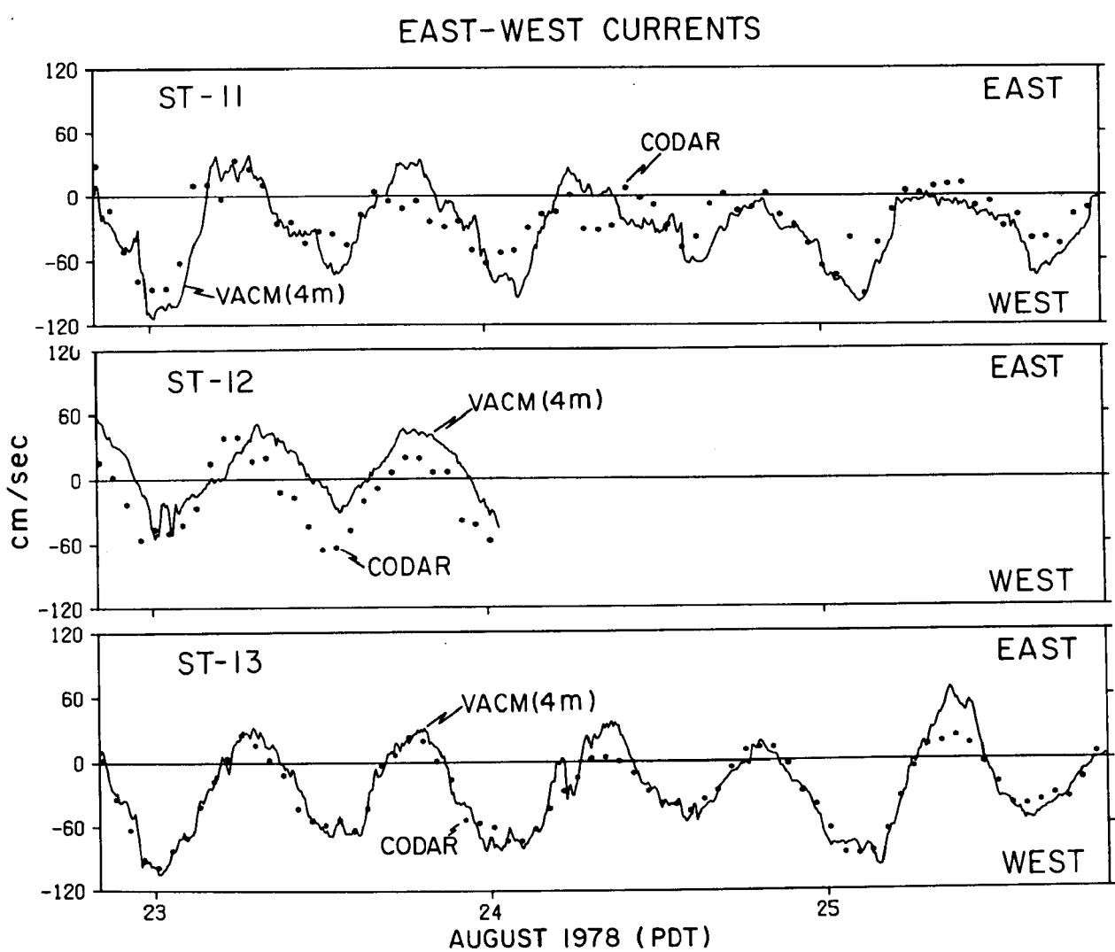
FIGURE 9.00. The radar measured current is compared with the current meter measurements at the four-meter depth for the east-west component.
