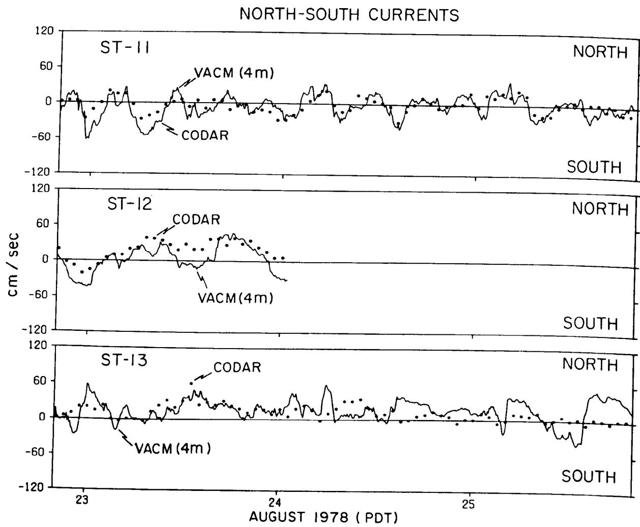
FIGURE 10.00. The radar measured currents are compared with the current meter measurements at the four-meter depth for the north-south component.
