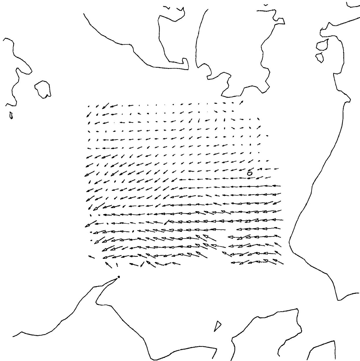
FIGURE 3a. Current maps generated from h-f radar observations. Radars were at New Dungeness Spit and Point Wilson. Asterisks denote the radar locations.
