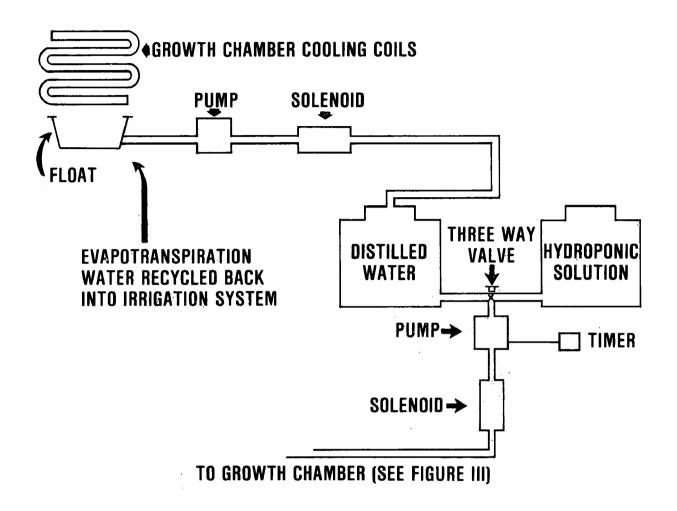
Figure 2. Schematic of the irrigation system used to recycle evapotranspired water, add nutrient solutions, and water plants growing in <sup>238</sup>PuO<sub>2</sub> contaminated soil.
