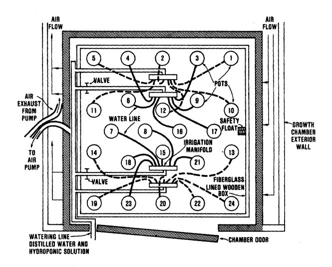
Figure 3. Design of the interior portion of the growth chamber showing the irrigation system, pot emplacement and direction of chamber air flow.
