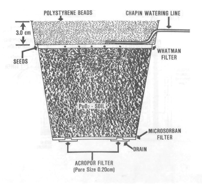
Figure 1. The design of five-inch plastic greenhouse pots used to hold the  $^{238}\mathrm{PuO}_2$  contaminated soil.
