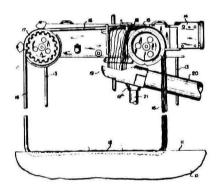
P-309-75 SCOOP FOR COLLECTING A LAYER OF POLLUTING MATERIAL ON WATER SURFACES
