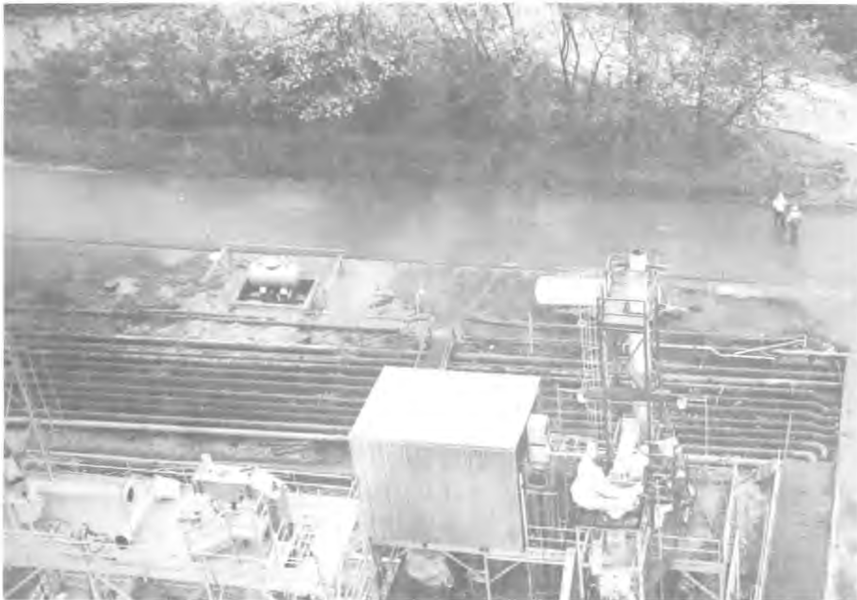
Figure 13. Operation with water wash ahead of first absorber stage.
