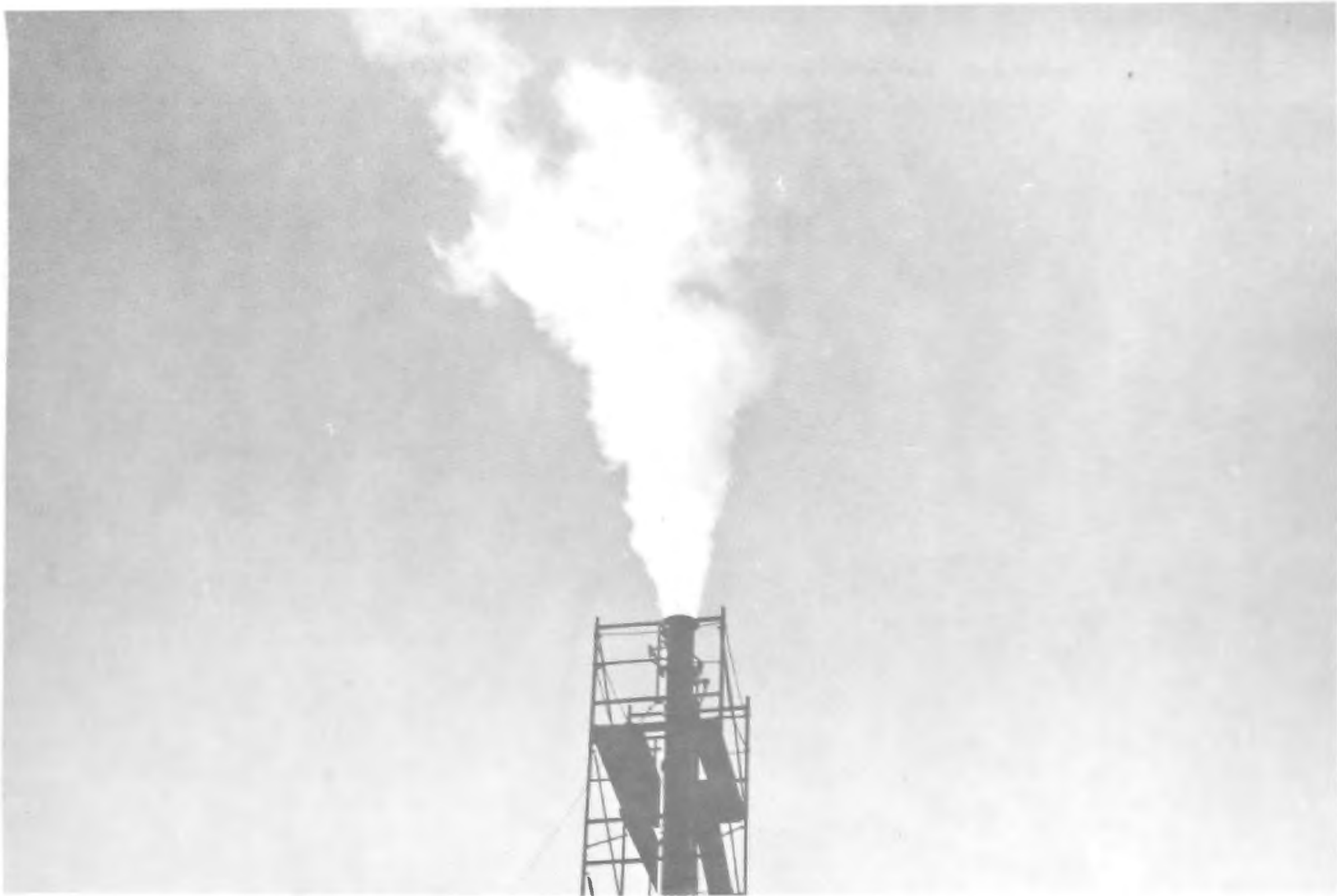
Figure 7. Plume from operation with scrubber solution having C = 1.0 ; no reheat.
