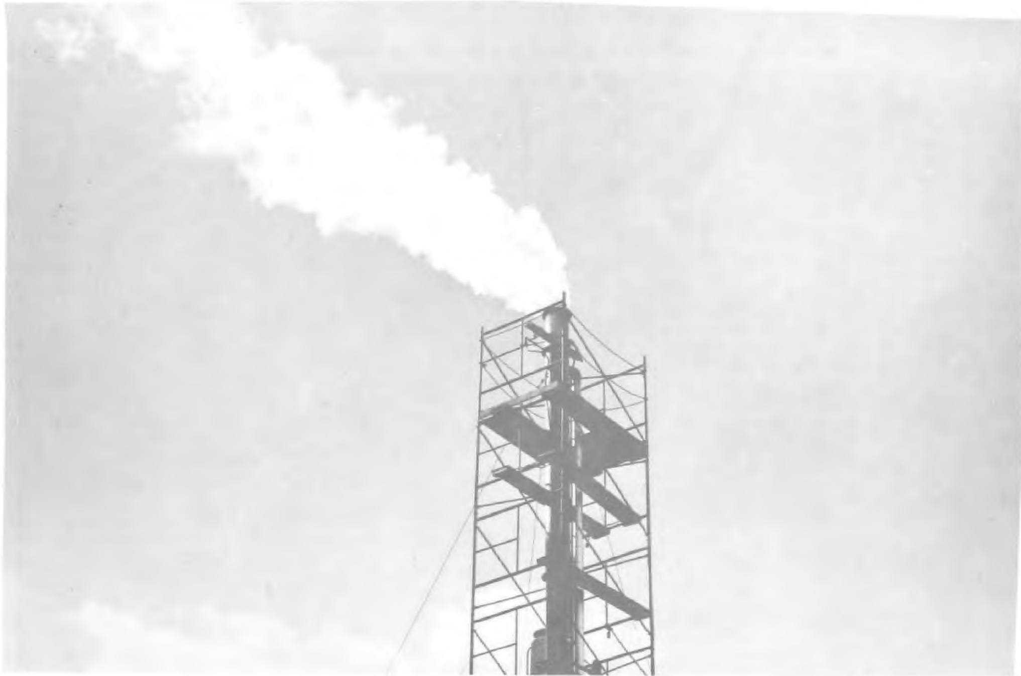
Figure 5. Plume emitted while scrubbing with water only; no reheat.
