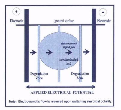
As illustrated in the diagrams, the outer layers consist of either positively or negatively charged electrodes. The electric field created by the electrodes moves contaminants in soil pore fluids into or through the treatment layers.
