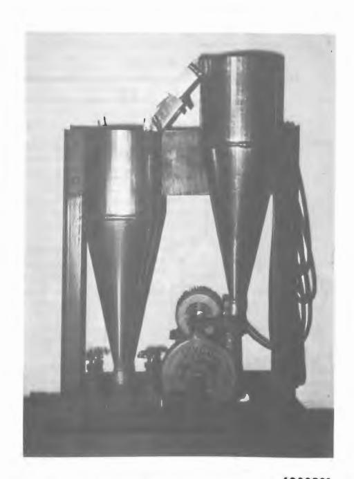
6082P21 Figure 2. Double Cone Heavy Media Separatory Unit
