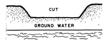
In a typical sanitary landfill, the maximum cut is made on the side slope. As the solid wastes are deposited, they are covered with the earth taken from the cut. This is continued until the site is filled. The entire area is then covered with a clean layer of earth. The final elevation depends on the planned use for the site.
