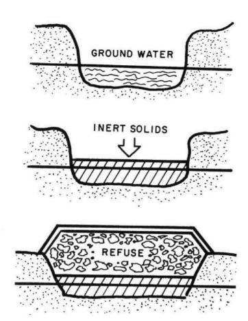
A pit site poses special problems if it has been excavated below groundwater level. It must first be filled with inert solids to a safe level above the groundwater before refuse can be deposited.
