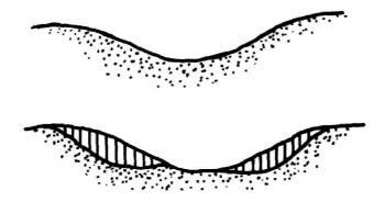
The maximum side slope cut possible in a valley or canyon is determined and the total volume of available earth calculated.
