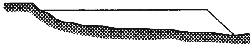
A valley-fill disposal configuration.
