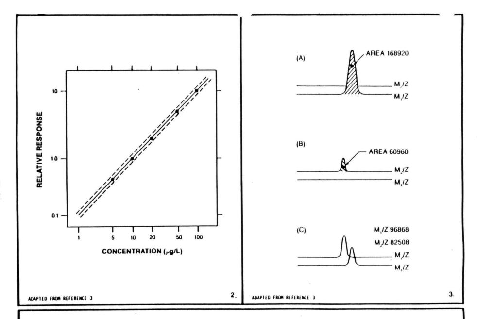
Figure II-2. Relative response calibration curve.
