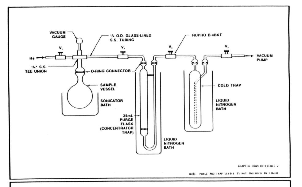
Figure II-1. Apparatus for vacuum distillation and cryogenic concentration.
