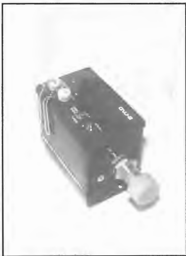
Figure 6. The ion mobility spectrometer sensor.
