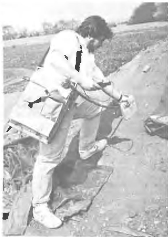
Fig. 1. FPXRF Analyzer X-MET 880 with a gas filled detector probe.
