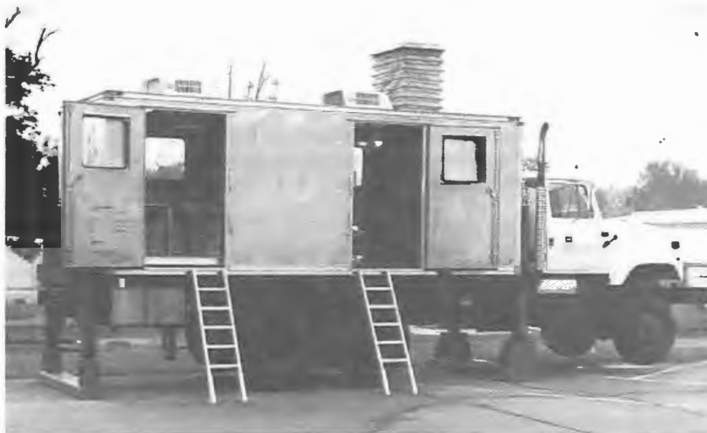
Figure 1. Photograph of penetrometer truck developed for use with the fiber optic fluorometer system. The data acquisition system and fluorometer system are located in the rear compartment. The hydraulic system used to push the penetrometer probe into the soil is in the forward compartment.
