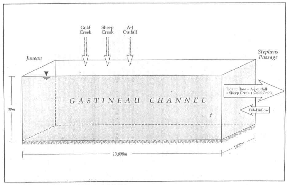
Figure 28 : Conceptual Diagram of Single Cell Model
