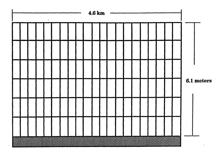
Figure 12. Two-dimensonal grid used for CE-QUAL-W2 simulations for tailings pond in Stage III. Nominal surface elevation of the pond is 279.5 meters above sea level.
