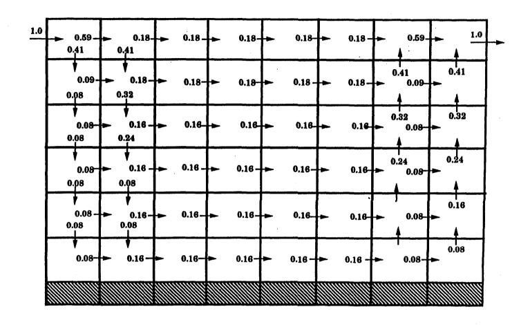
Figure 9. Velocity profiles used for uniform flow scenarios in the WASP4 analysis of the proposed AJ Mine tailings pond. Numbers by arrows indicate fraction of total flow.
