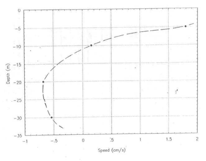
Figure 27: Residual along-channel velocity profile for period 18 February to 24 April 1992
