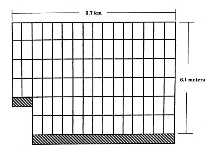
Figure 11. Two-dimensonal grid used for CE-QUAL-W2 simulations for tailings pond in Stage I. Nominal surface elevation of the pond is 233.0 meters above sea level.
