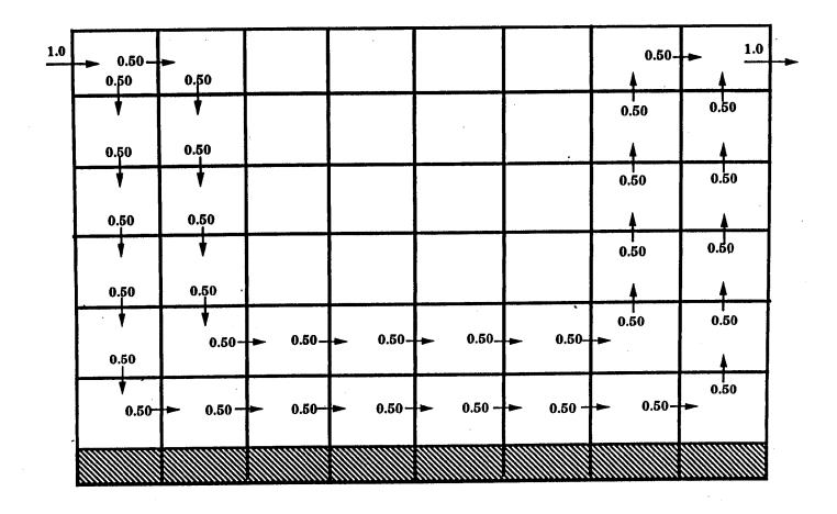
Figure 10. Velocity profiles used for underflow scenarios in the WASP4 analysis of the proposed AJ Mine tailings pond. Numbers by arrows indicate fraction of total flow.
