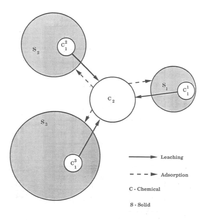
Figure 5. Conceptual model of geochemical processes for metals in the proposed AJ Mine tailings pond
