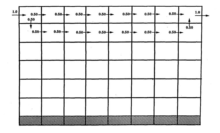
Figure 8. Velocity profiles used for surface flow scenarios in the WASP4 analysis of the proposed AJ Mine tailings pond. Numbers by arrows indicate fraction of total flow.
