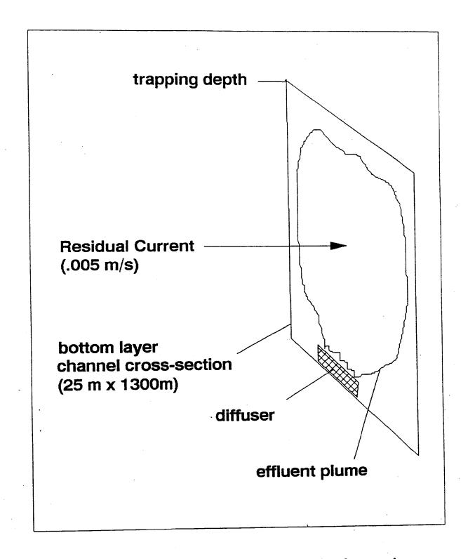
Figure 29: Conceptual Framework for Volume Flux Approach
