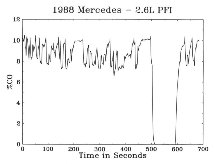
%CO data collected with a 4 gas analyzer from a 1988 Mercedes Benz 190E over a road course of stop-and-go/freeway driving. Low emissions are observed when presumably the oxygen sensor was functioning properly.
