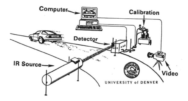
A schematic diagram of the University of Denver on-road emissions monitor. It is capable of monitoring emissions at vehicle speeds between 2.5 and 150 mph in under one second per vehicle.
