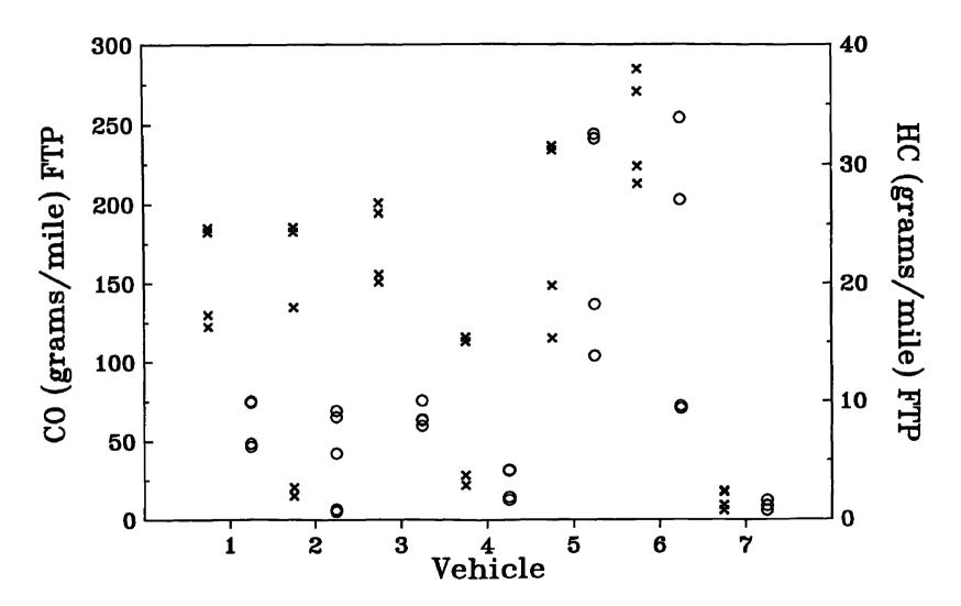
FTP data for CO and HC emissions from seven 1986 and newer model year high emitters. Four (or 5) separate tests on the same fuel are plotted for each vehicle for CO (x) and HC (o).
