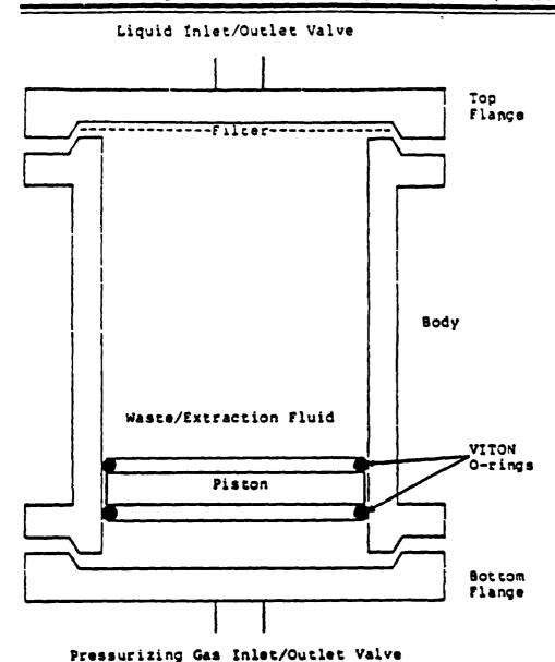
Figure 3: Zero-Headspace Extraction Vessel
