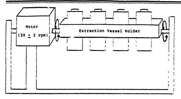
Figure 2: Rotary Agitation
