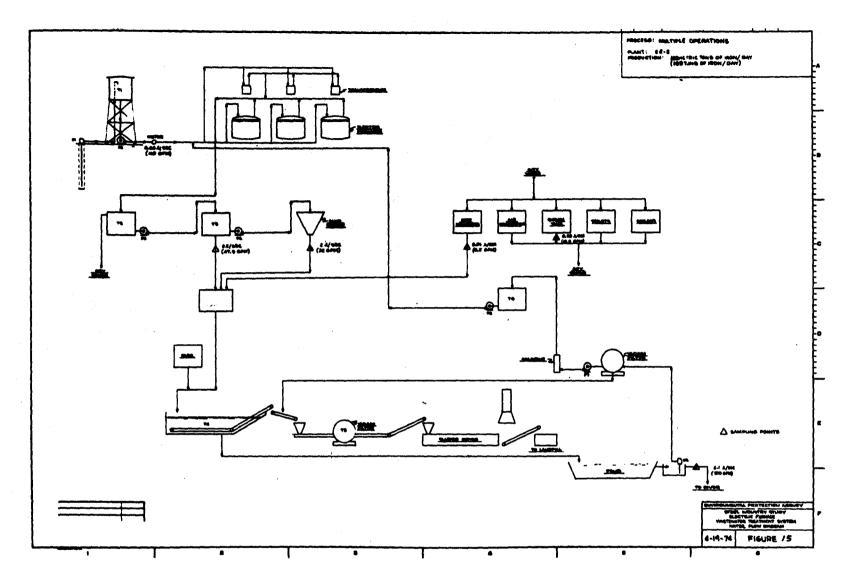
flocculant and proceeds through a settling basin. Solids are removed at about 25% and processed through a vacuum filter to achieve 50 to 60% solids. These are next processed through a dryer and then sent to landfill at about 95% solids.
