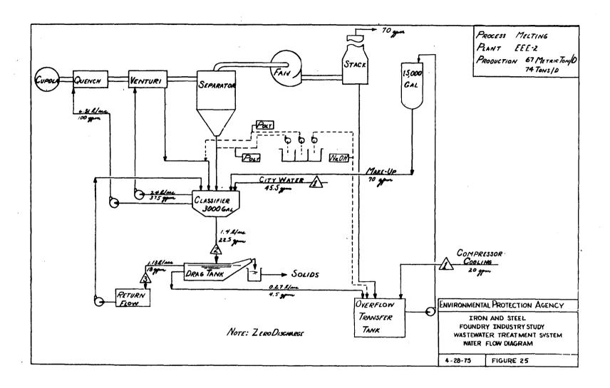
The overflow tank collected noncontact cooling water from the air compressors, and pumped it and the drag tank overflow water to a head tank for makeup to the system. Caustic was also added at this tank for corrosion control.
