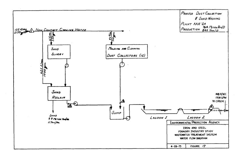
The lagoons were arranged to give maximum use of the land area. The inlet to the first lagoon was arranged so that the heavy solids could be removed readily. This was a daily routine.
