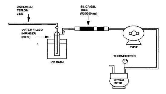
Figure 308.1. Sampling train schematic
