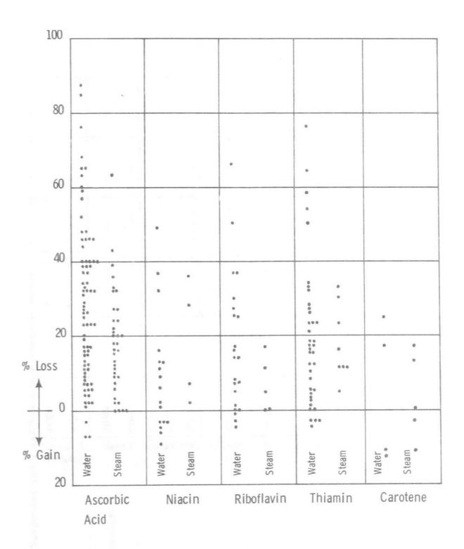
Figure 3. Losses in Vitamin Content of Fruits and Vegetables from Water and Steam Blanching
