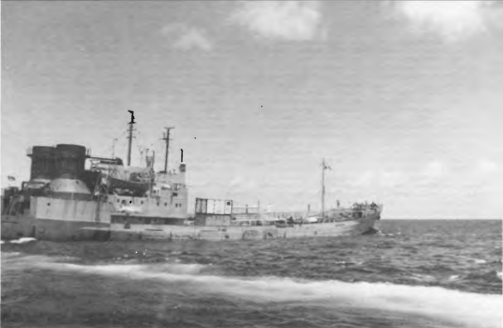
Twin chimneys at the stern of the Vulcanus mark the location of the incinerator, which destroys toxic substances by burning them at extremely high temperatures.
