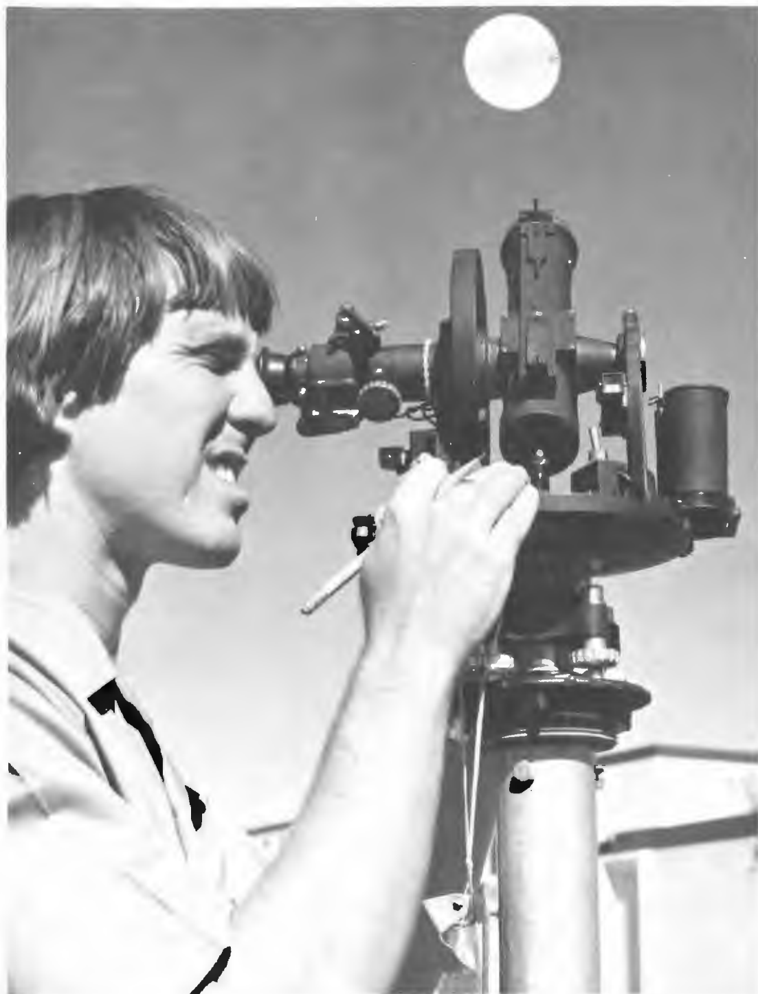
EPA scientists plot wind direction and speed in air pollution studies by tracking a helium-filled balloon with this instrument, a theodolite.
