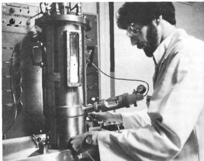
A researcher uses a fermenter to grow bacteria which have been genetically engineered to produce larger quantities of proteins or chemicals for use in scientific studies.
