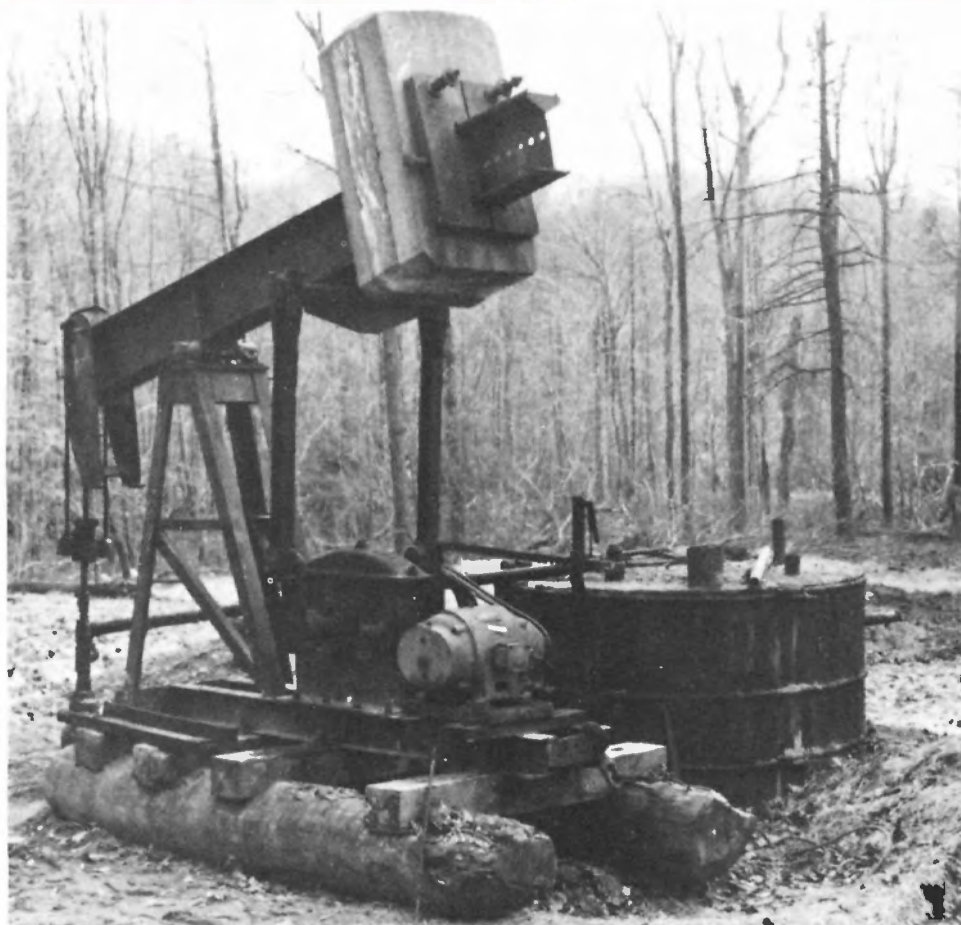
A typical oil production operation in northwestern Pennsylvania, with oil well, jack, and stock tank.
