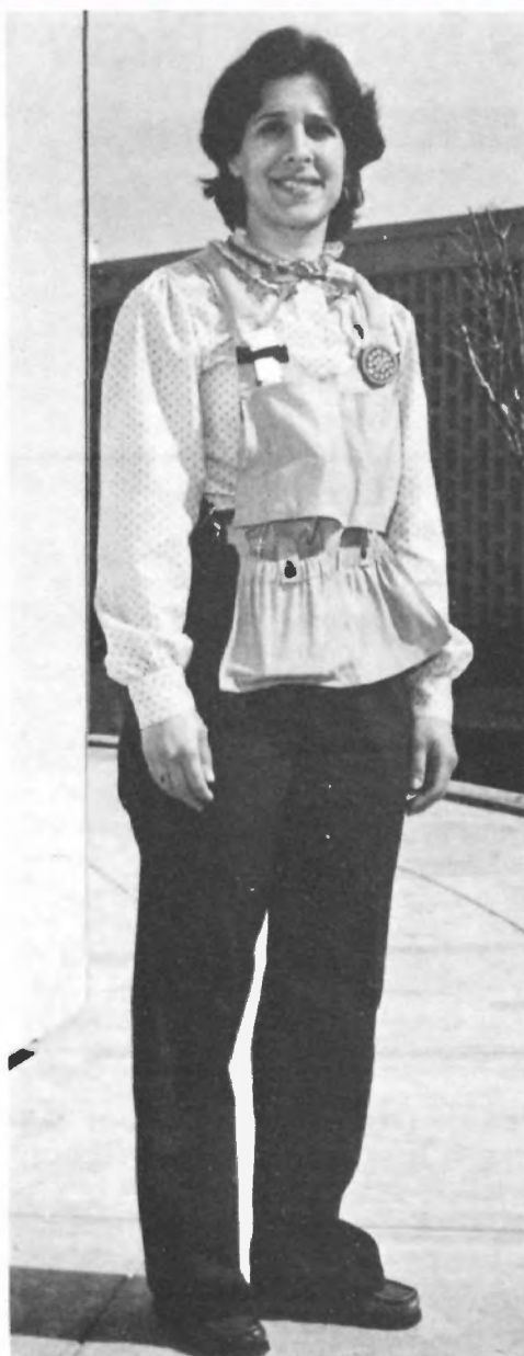
Patricia Blau of Research Triangle Institute, a non-profit contractor for EPA, wearing a specially designed vest containing a personal air monitor and a battery-powered pump for collecting air samples.
