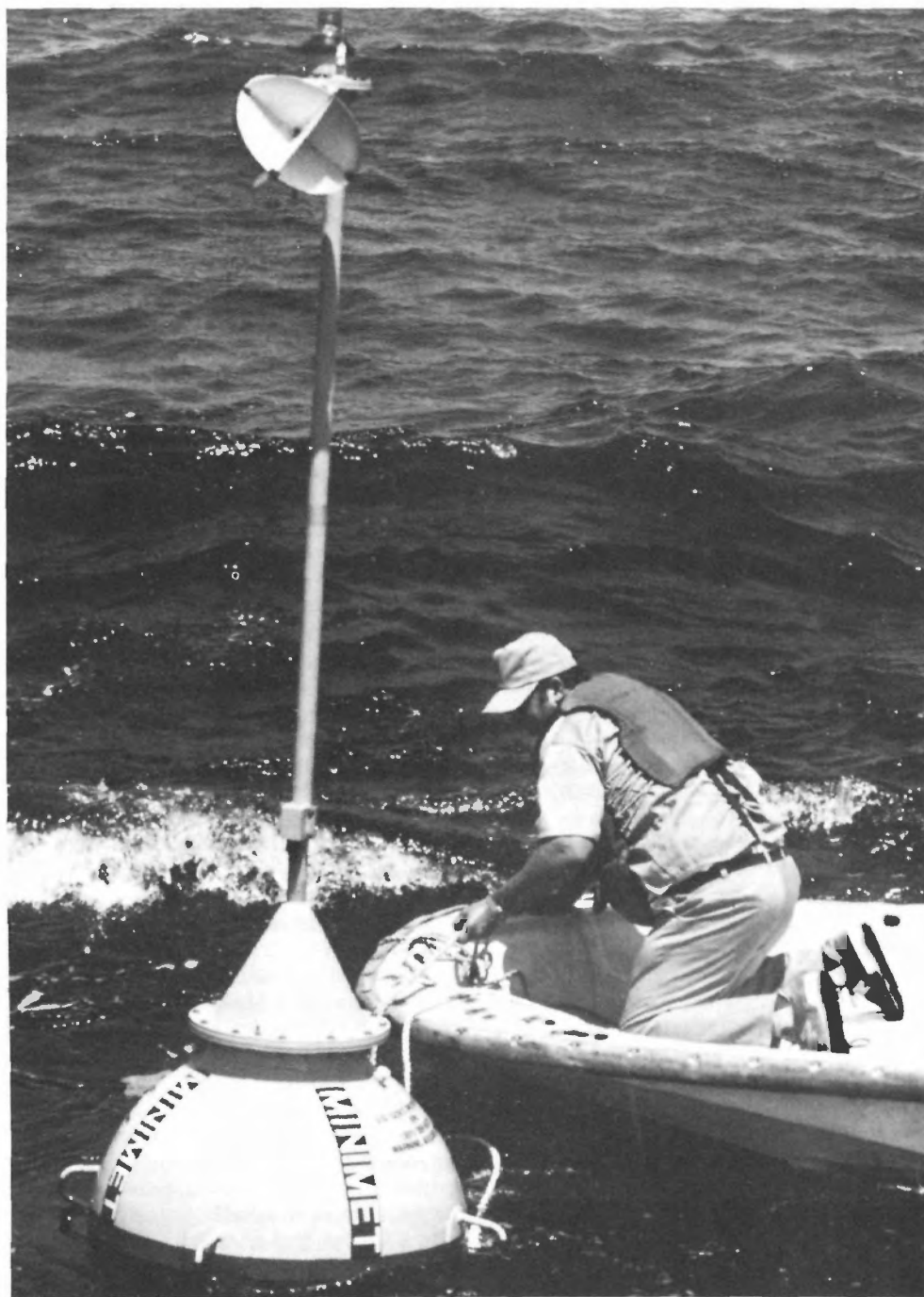
EPA's ship, Peter W. Anderson , currently located in the Chesapeake Bay, does marine research and monitoring. From a dinghy, crew member Robert Orme checks a buoy which radios data on water temperature, salinity, and dissolved oxygen back to the EPA liaison office in Annapolis, Maryland. Steve Delaney photo.
