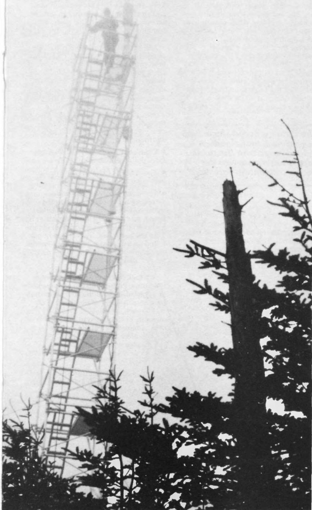
A man-made spider web of teflon string sits atop a tower on Mt. Mitchell in North Carolina's Mt. Mitchell State Park. As clouds roll in, cloud droplets deposit on the teflon strings. Slowly, the water drips off the strands of the web and into a small trough. Every hour, a man climbs up the 70-foot tower and empties the trough. He climbs other towers to empty other troughs. Whenever clouds appear he performs this ritual.
